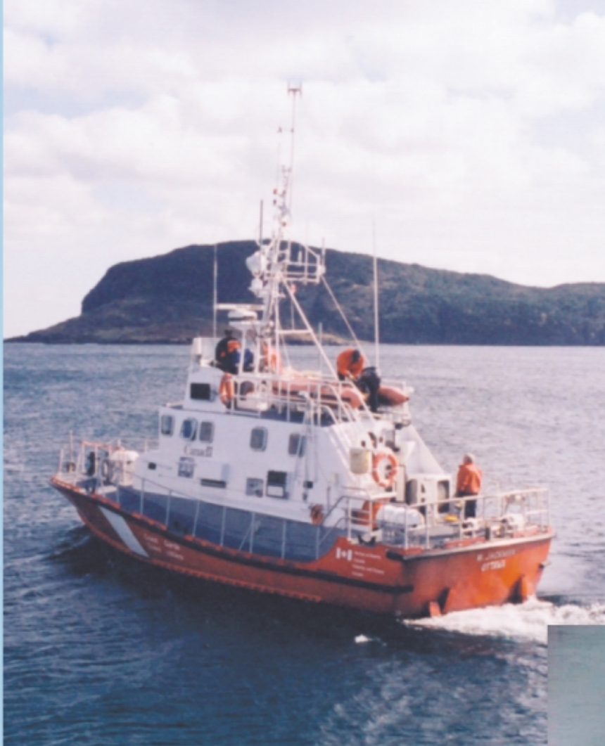
An Arun Class Cutter such as the CCG W. Jackman offers high speed, high endurance rescue capabilities
