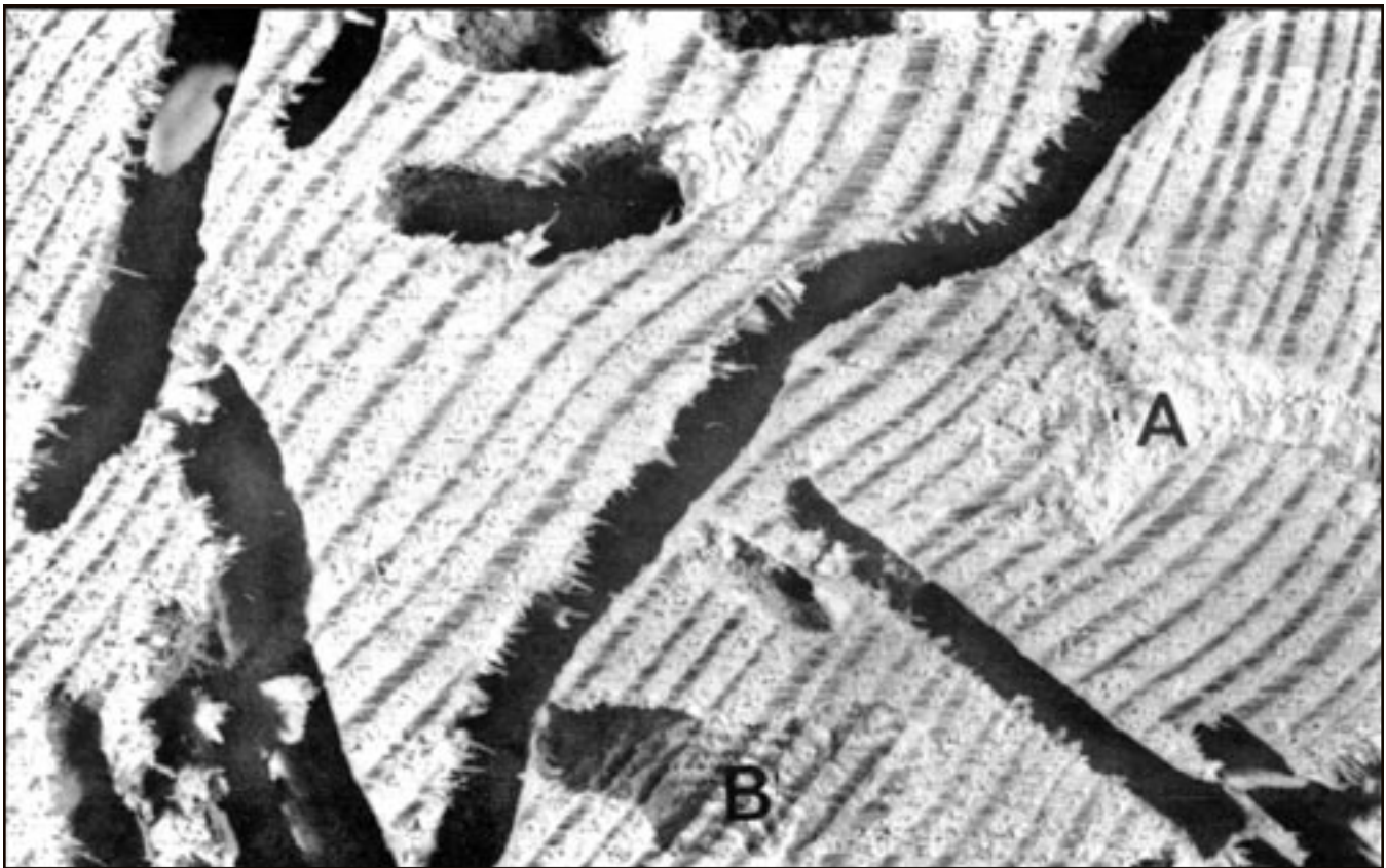
Figure 3. Cross section of larval tunnels. A. Larval tunnel packed with frass. B. Fine grooves on wall of tunnel.
