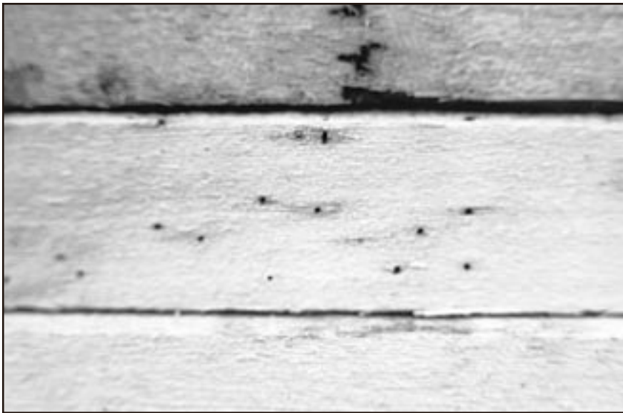
Figure 2. Lumber showing ambrosia beetle entrance holes (pinholes) which result in degrade.
