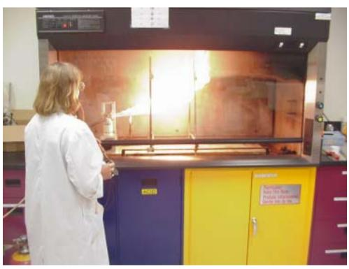
Flame projection and flashback testing of aerosol containers
