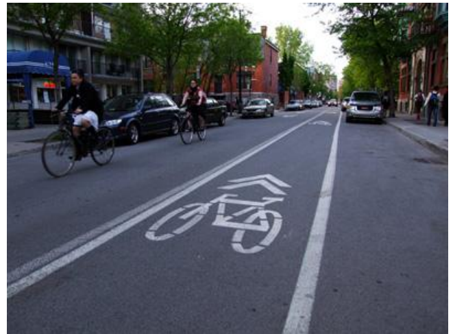
Figure 2. Contra-flow bicycle lane in Montreal allows cyclists to travel in the direction opposite to traffic on a one-way street (photo: Christopher DeWolf)
