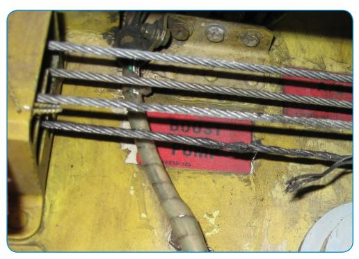
A reminder for personnel that during flight control cable inspection that the entire cable run must be inspected to detect these types of failures. \*
