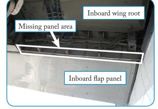
Aviation Safety Agency Airworthiness Directive 2008–0002 was issued mandating the incorporation of Service Bulletin A330–57–3100, which replaces the existing blind rivets with bolted fasteners.
