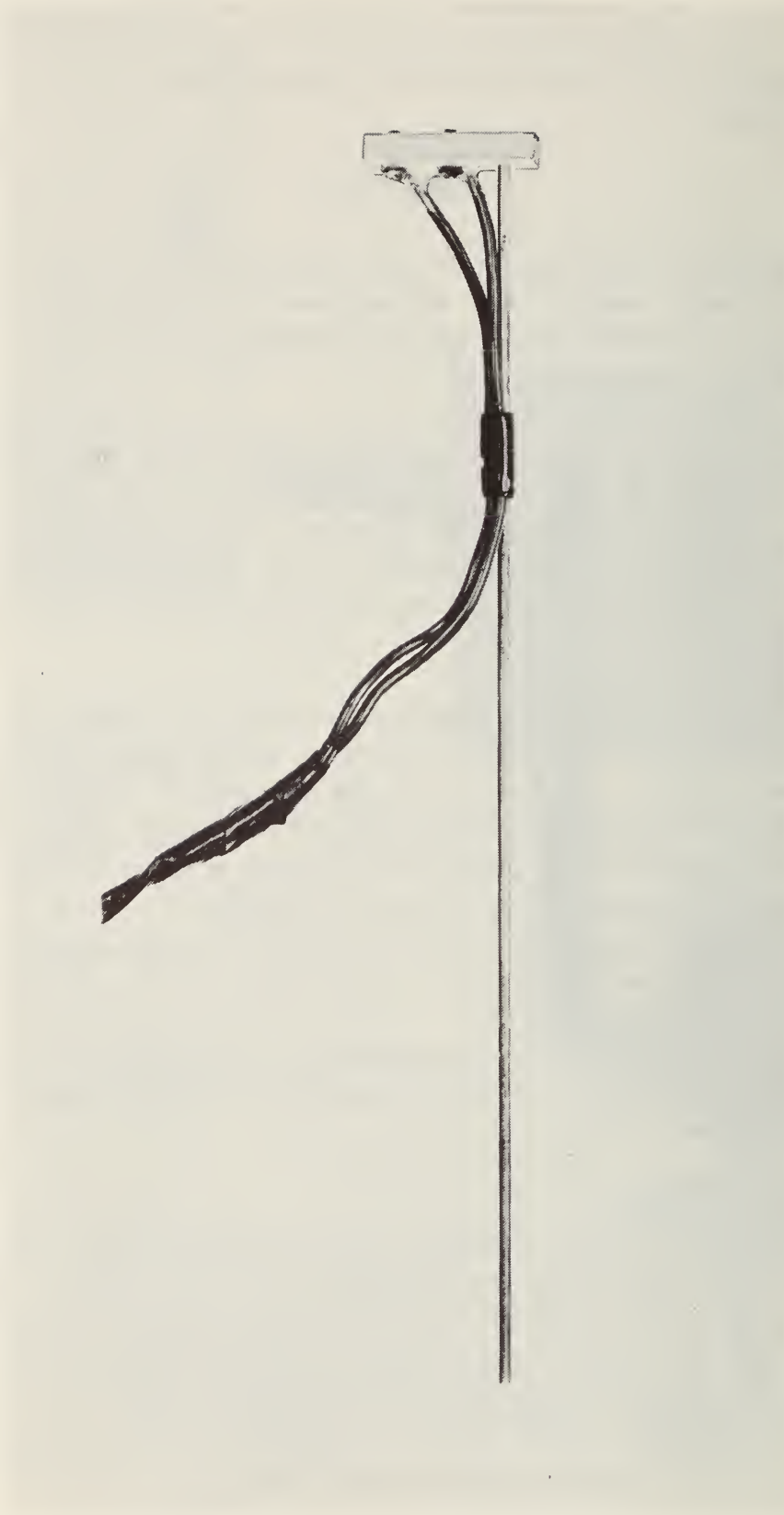
Figure 7.— An electronic leaf control. Leads are attached to a relay switch that operates a solenoid valve.
