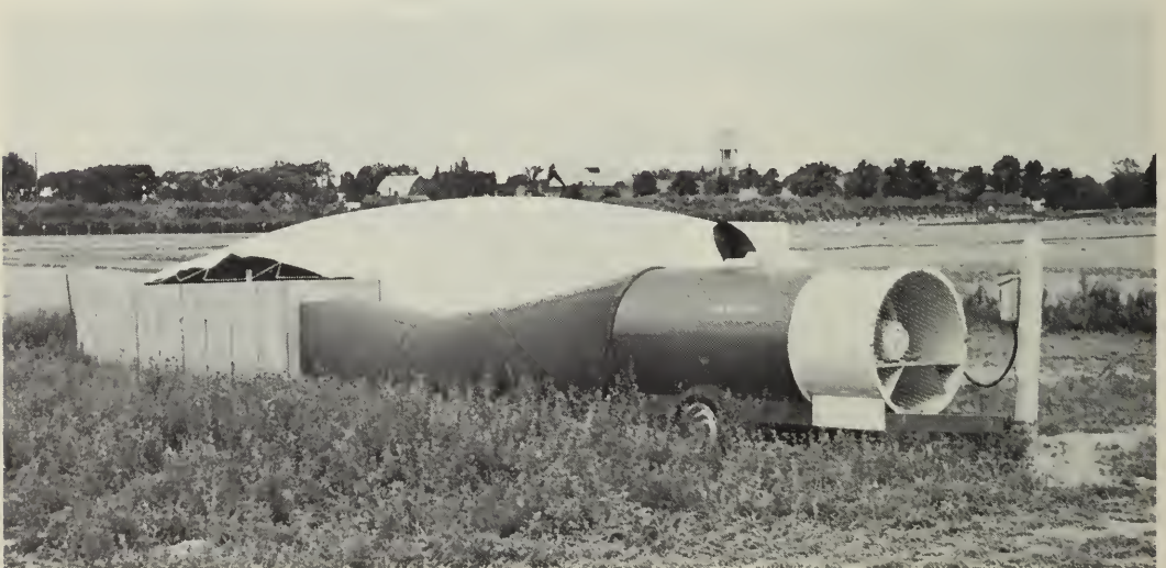
Oil-fired gun-type heating unit with heat exchanger attached to duct and tarpaulin-covered drying box.
