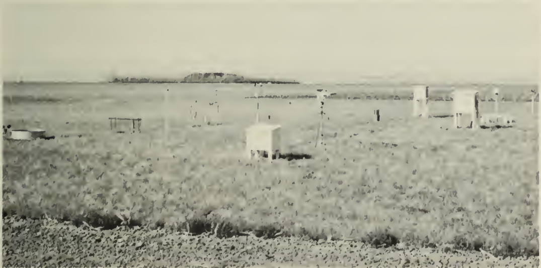
The agrometeorological observation site at Swift Current, Saskatchewan. The instruments are, from left to right: United States Weather Bureau Class A evaporation pan with a totalizing anemometer set at 18 inches; Canada Department of Agriculture Experimental Farm 4-foot buried tank with screen; black Bellani plate evaporimeter with mercury valve; black porous disc evaporimeter; recording anemometer with direction vane; power outlet (in foreground); standard 3½-inch rain gauge; Nipher shielded precipitation gauge; Suomi ventilated net radiometer (in foreground); tipping bucket recording rain gauge; Stevenson screen; junction box for wiring terminals with asbestos conduit leading to recorders in field building; Eppley pyrhelimeter; Campbell-Stokes sunshine recorder.
