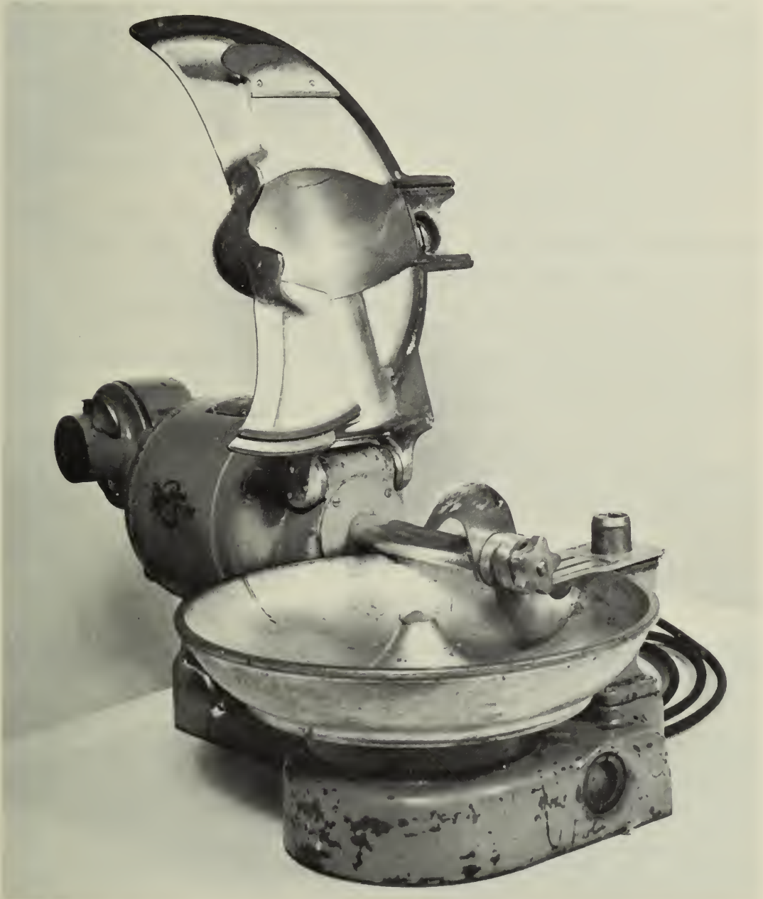
Salad chopper used to chop and mix fresh herbage or silage. More accurate sampling is possible following this technique of preparation.
