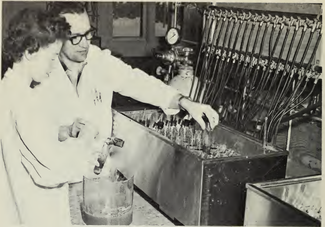
A continuous-gassing in vitro system, showing manifold (upper right) and water bath
