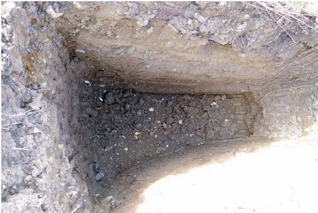
Test Pit for Ground Disposal
