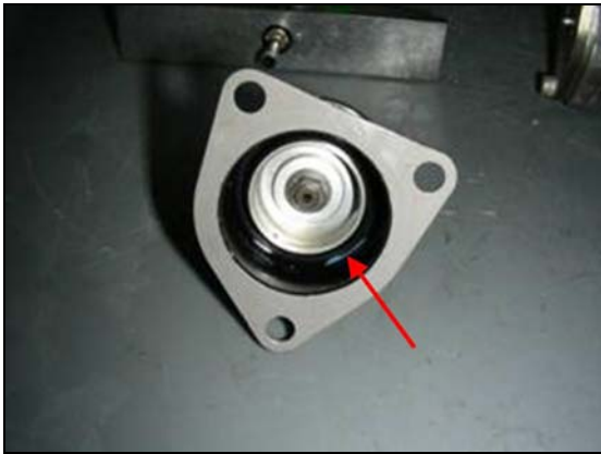
Photo 3. Debris in delta P diaphragm chamber
