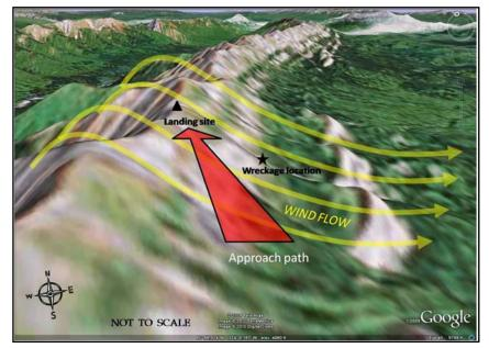
Figure 1. Flight path and wind flow
