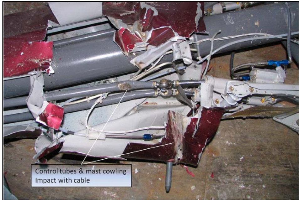
Photo 1. Cable marking on control tubes
