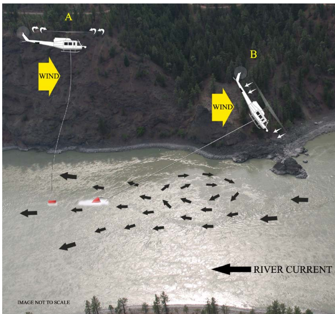
Figure 2. Accident sequence (VRS followed by bucket anchoring)
