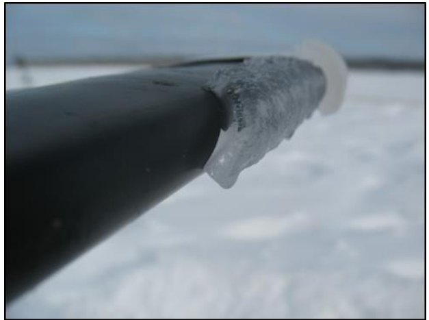
Photo 4. Ice on the horizontal stabilizer leading edge
