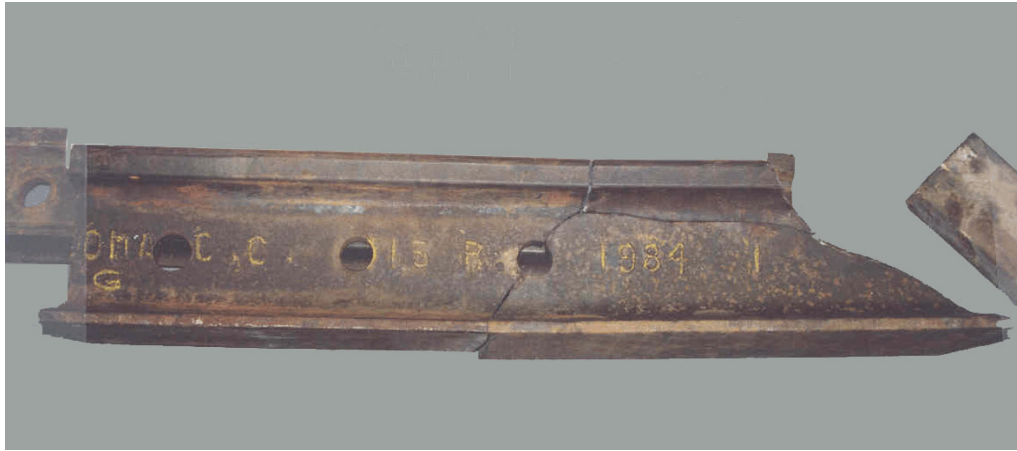
Photo 1. Reconstructed rail from suspected POD
