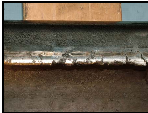
Photo 8. Gauge face of rail showing indications of scuffing and tearing
