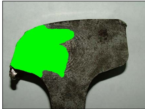
Photo 7. The burnished fatigue area (green) of fracture surface A
