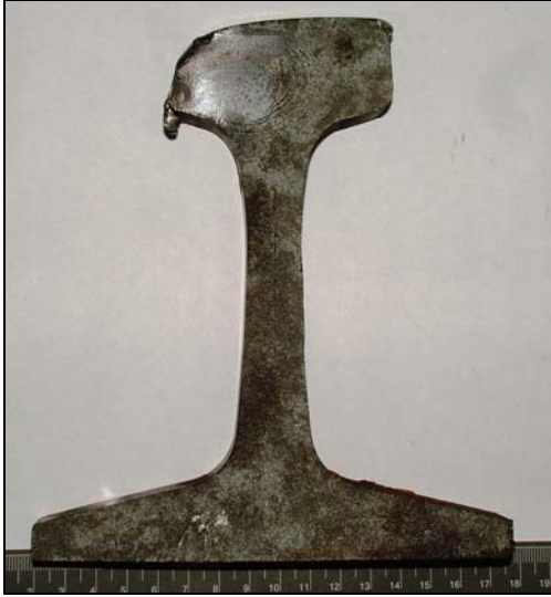
Photo 2a. Face de rupture A
