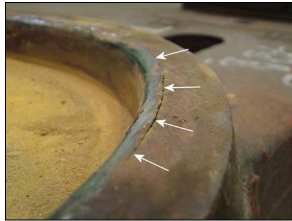
Photo 6. Edge of truck centre plate with raised lip that was smeared from contact wear
