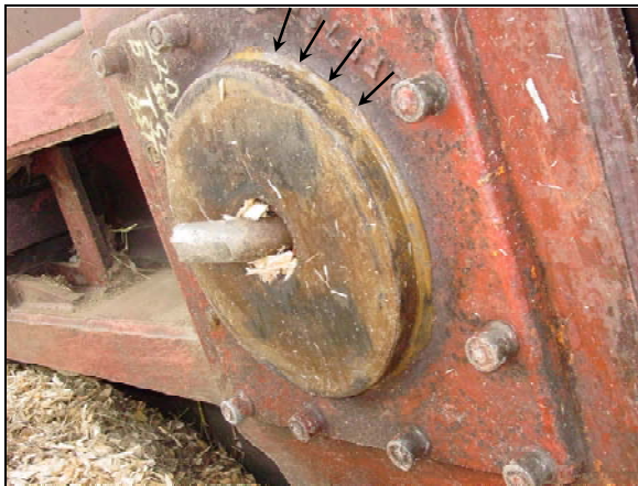
Photo 5. Body centre plate (B-end). Arrows point to wear area
