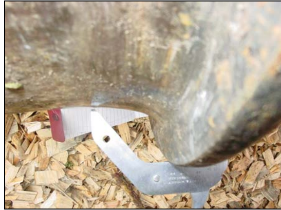
Photo 4. High-flange condition on one wheel set
