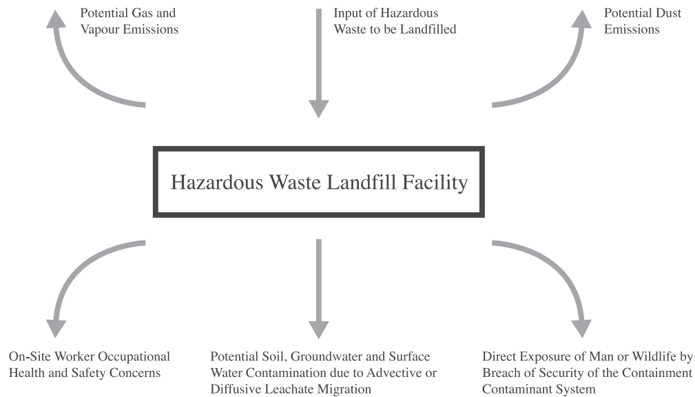
Figure 1. Schematic diagram of potential release pathways for material from a hazardous waste landfill.
