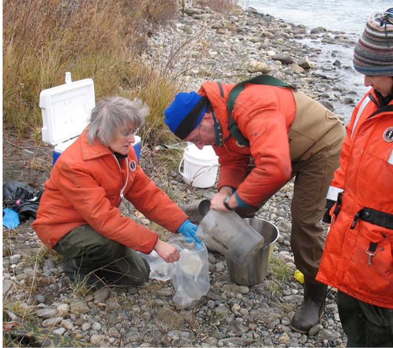
Photo 14. Transferring sediment samples to containers (Courtesy: Darcy McDonald Alberta Environment)
