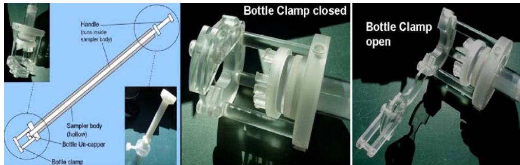
Photo 11. ISOMET sampler (Source: Environment Canada (2008 draft))
