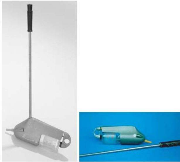
Photo 16. Manual suspended sediment sampler on sampling rod
