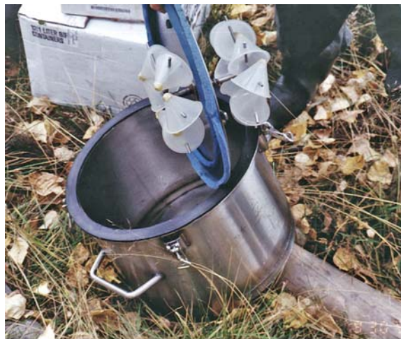
Photo 17. SOD chamber (Alberta Environment (2006a))
