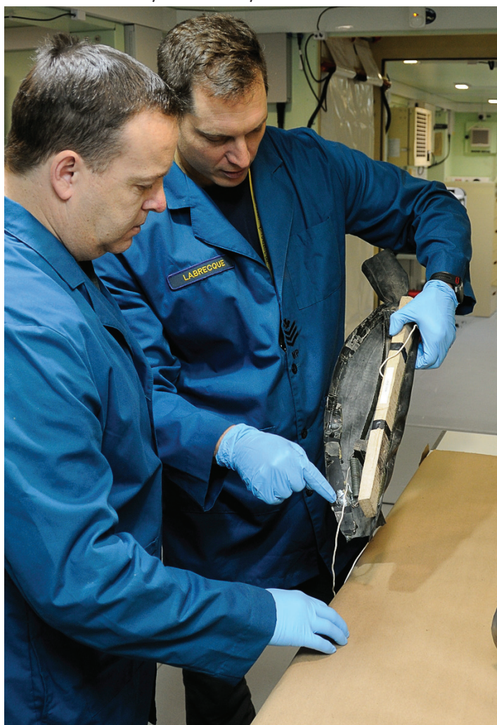
Sergeant Carl Labrecque and Master-Corporal J.P.R. Tremblay conduct forensic procedures on a pressure plate used by insurgents in Afghanistan to detonate Improvised Explosive Devices
