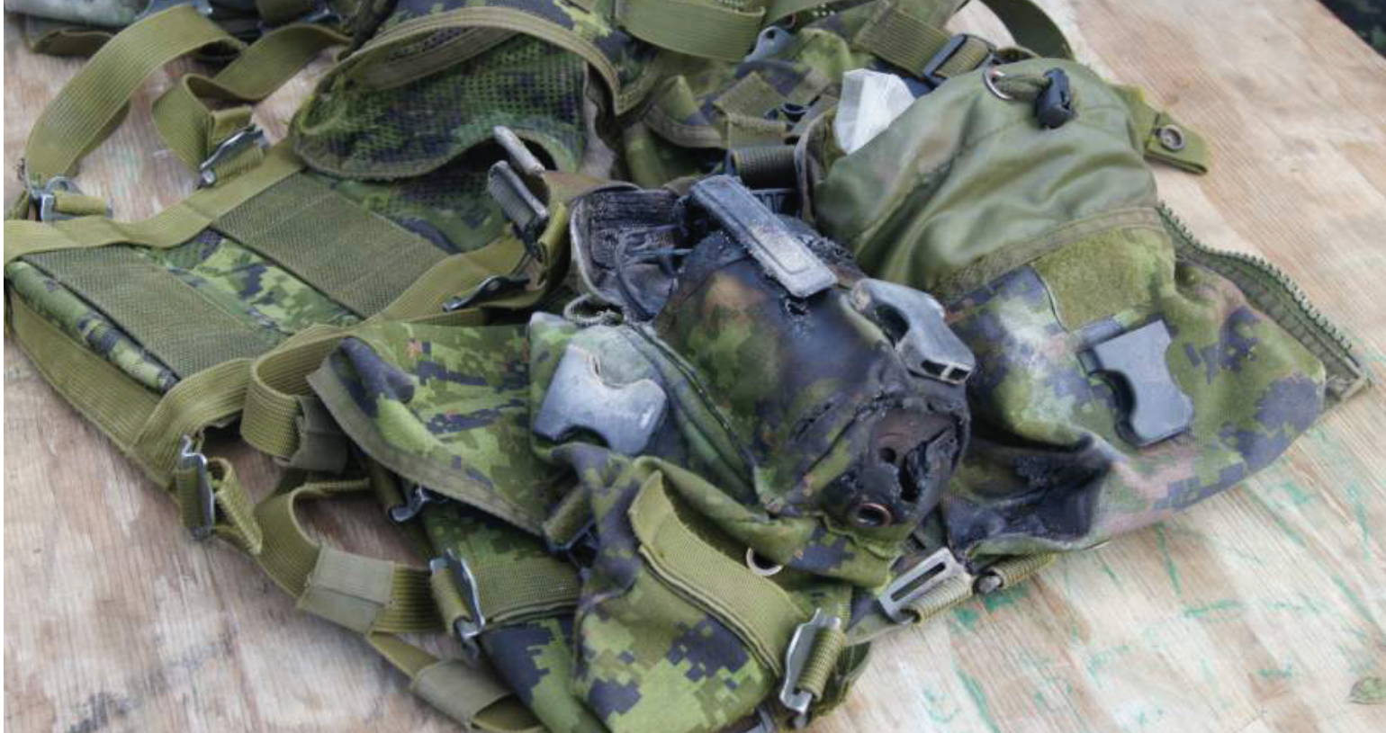
Tactical Vest damaged by an L83 smoke grenade that was initiated as a result of the fly up lever getting caught in its surroundings
