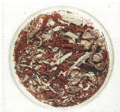
Figure 1. Sealant Material Found at the Bottom of Tank
