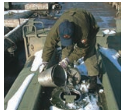
Figure 3. Improper Method to Add FSII
