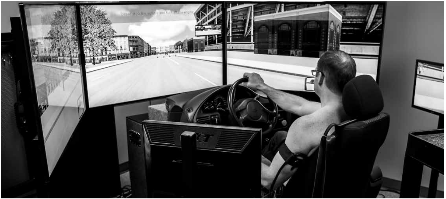
The Healthy Driver Research Group uses driving simulators to test reaction times and other cognitive performance measures following a night shift.
