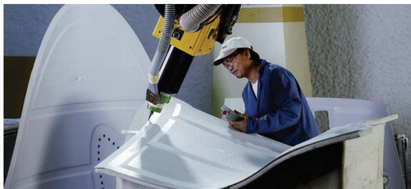
5-axis machining of composite structures — Magellan
