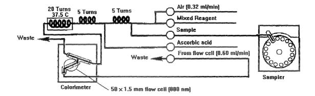
Figure 7. Flow diagram for phosphate analysis.
