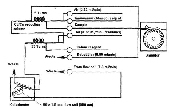
Figure 8. Flow diagram for nitrate analysis.
