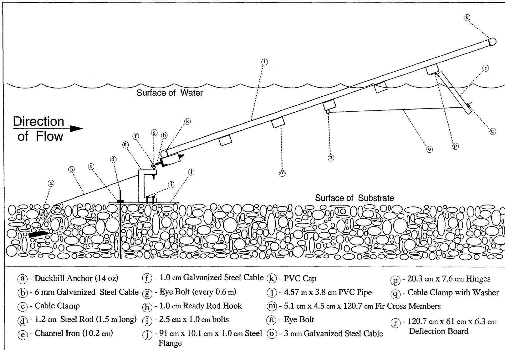
Figure 2. Diagram showing a PVC conduit panel and the channel iron anchoring system (cross-sectional view).
