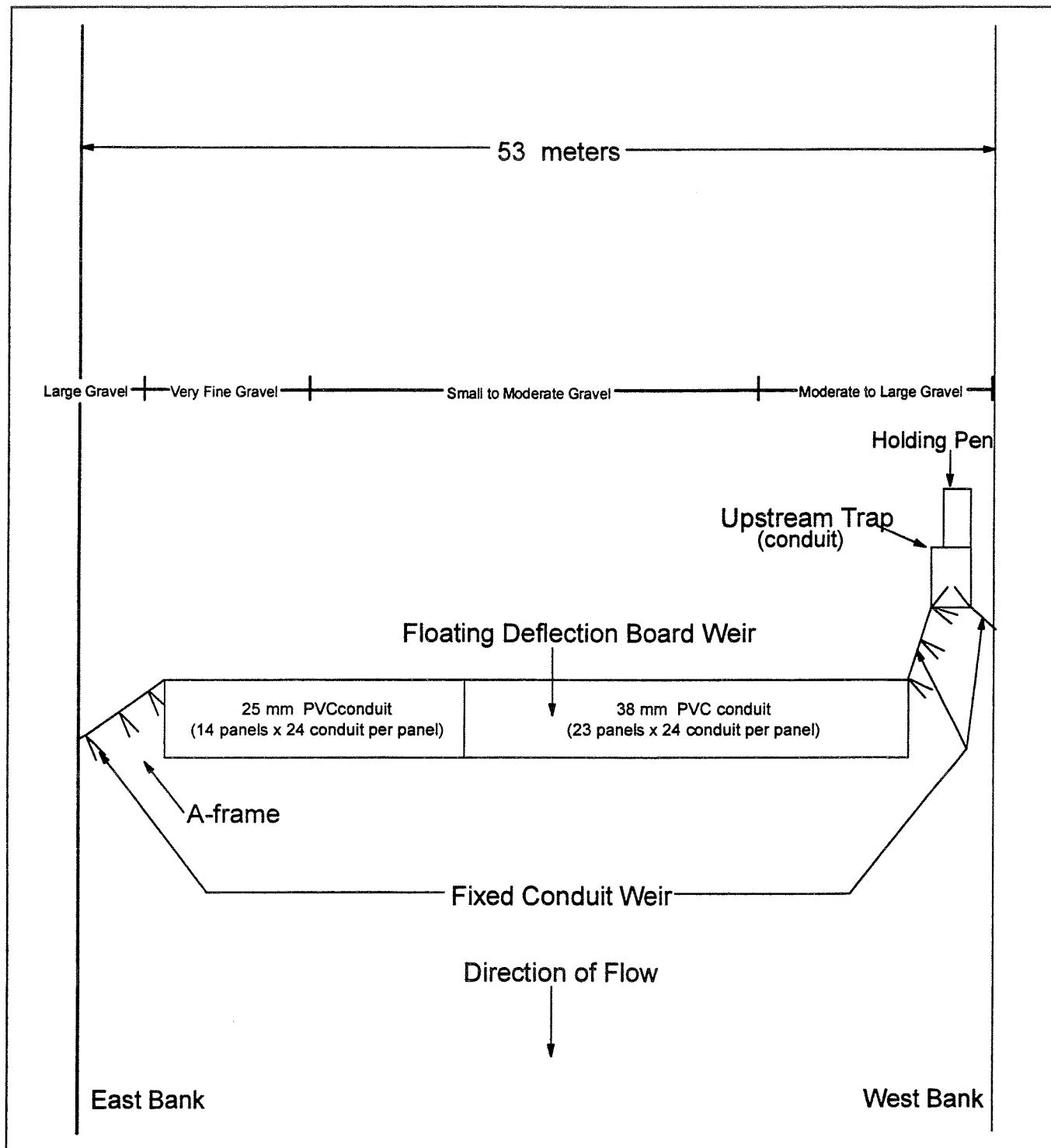
Figure 6. Configuration of the 1992 floating deflection board weir on the Babbage River.
