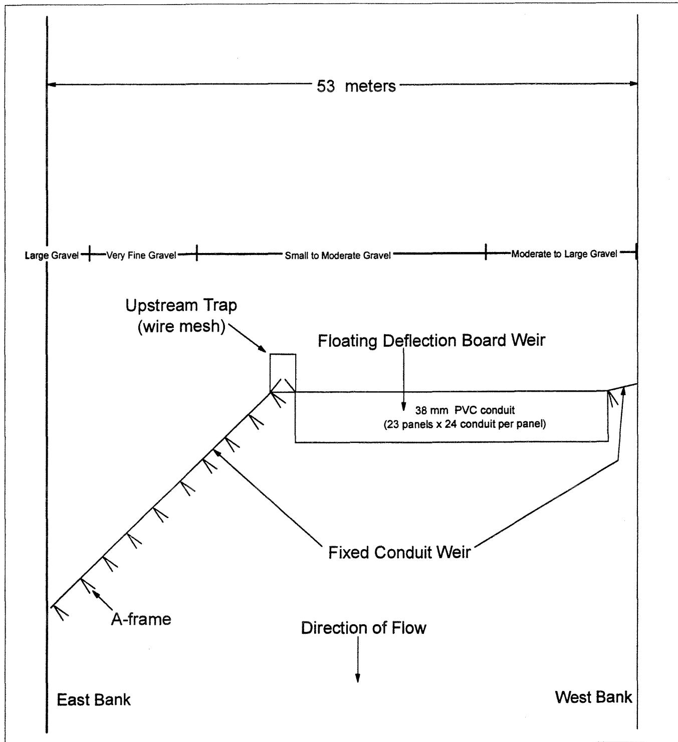
Figure 4. Configuration of the 1990 floating deflection board weir on the Babbage River.
