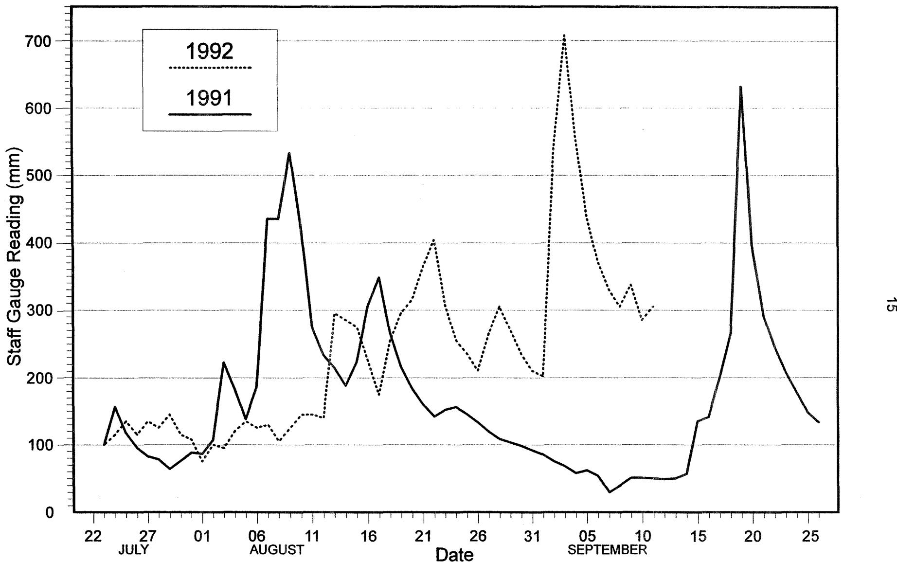
Figure 10. Average daily staff gauge (i.e., water depth) measurement (mm) recorded in 1991 and 1992 at the weir on the Babbage River. The 1991 and 1992 recordings were not standarized between years, thus recordings only represent actual change in water depth within a given year.
