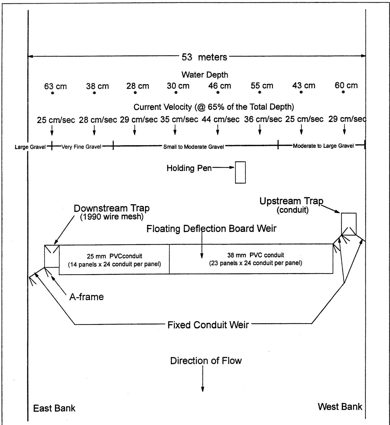
Figure 5. Configuration of the 1991 floating deflection board weir on the Babbage River. Depth and current profiles were recorded on August 1<sup>st</sup>, 1991 at a staff gauge reading of 325 mm.
