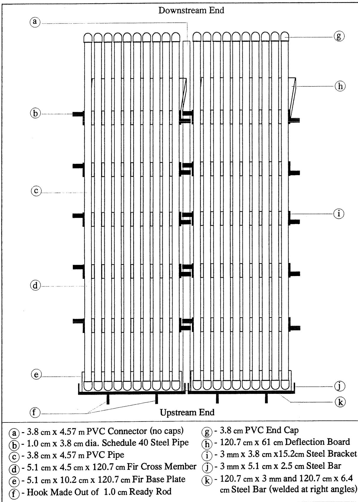
Figure 3. Diagram of two PVC conduit panels (top view). Each panel is depicted with only 10 PVC conduit to reduce the required space for the drawing. In actuality each panel contained 24 individual PVC conduit.
