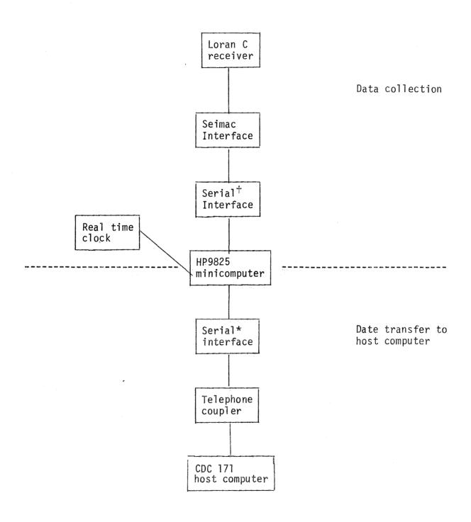
†baud rate: 2400 (setting = 3) \*baud rate: 300 (setting = 7)
