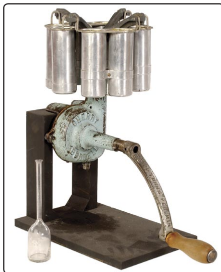
This Babcock tester, supplied by Ketchum Manufacturing of Ottawa, was used in the dairy technology laboratory at the Central Experimental Farm (790290).
