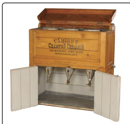
The top of the Champion Cabinet creamer was filled with cold water to speed the separation of milk and cream. Once separated, the milk was drained off through the valve at the bottom of each of the three cans contained in the cabinet (730341).
