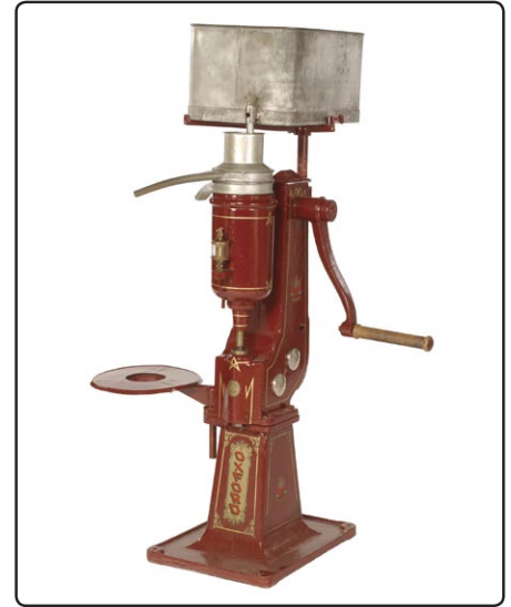
The cream separator's bowl, spouts and disks all had to be washed in hot water after each use to remove rancid milk that might contaminate the next batch (D2780 3012C).
