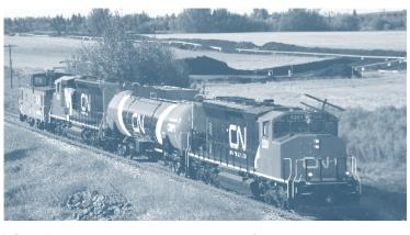
The Transport Dangerous Goods Directorate issued an Equivalency Certificate to Canadian National Railways (CN) to allow them to use an experimental tender in a pilot project that uses new liquefied natural gas technology to fuel locomotives. Ön September 27, 2012, CN announced that it was testing two mainline dieselelectric locomotives fuelled principally by natural gas. These locomotives will run on the 480 km line from Edmonton to Fort McMurray, the rail gateway to the
