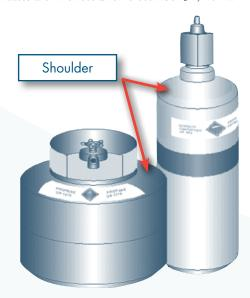
After December 31, 2014, no reduced labels will be allowed on the cylindrical part of cylinders. In the meantime, Transport Canada will review *Transportation of Dangerous Goods Regulations* requirements, to allow reduced labels on cylinder shoulders.
