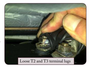
Extensive trouble shooting was carried out with no faults found. The left-hand power junction box was again replaced with nil fix. While removing the right-hand power junction box for replacement, the two rear connections at Terminal 2 and Terminal 3 were found to be significantly loose and arcing on the lugs.
