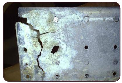
panels to the rear floorboards will then allow maintenance personnel to conduct a thorough corrosion related inspection of this important area. Additionally, TCCA recommend that operators also comply with the inspection procedures outlined in Piper SB 789A.
