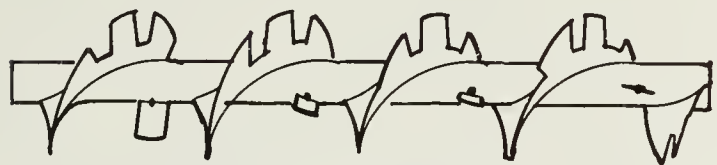
CUT FLIGHTING with PADDLES High Degree of Mixing and Aeration for Material in Transit
