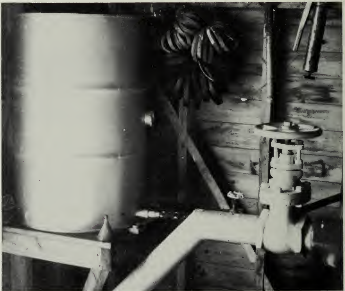
FIGURE 22 The insecticide is mixed in the barrel shown here and applied through the irrigation system.
