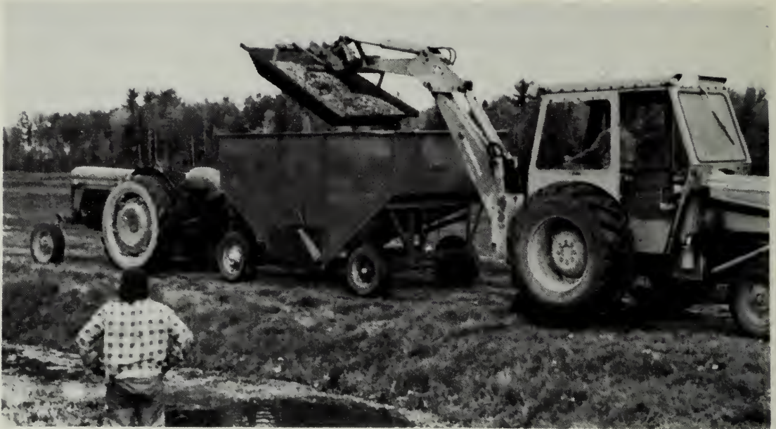
FIGURE 10 Boats containing cranberries are transferred from the bog to the wagon by a forklift and then the berries are transported to a packing plant. A drain at the bottom of the wagon allows excess water trapped in harvesting to be released.
