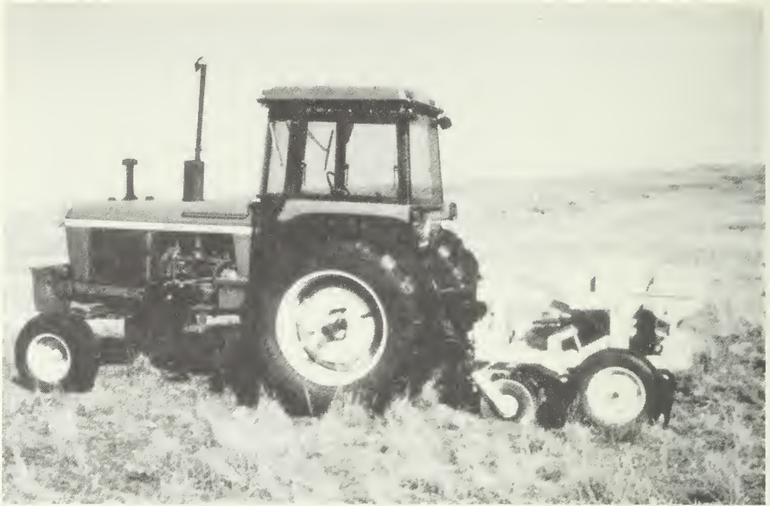
Fig. 6 Truax rangeland seed drill suitable for seeding grasses and legumes.
