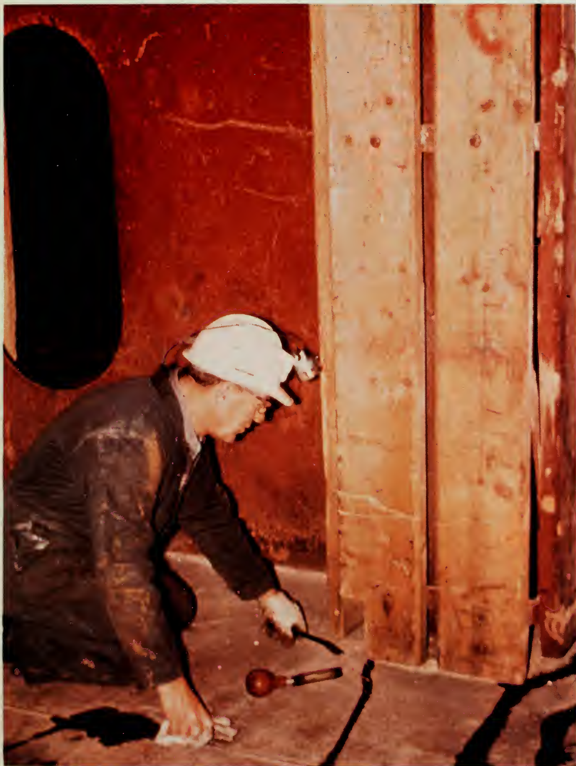
Examining the base of a pipe casing, where grain may accumulate and insect infestations may occur.
