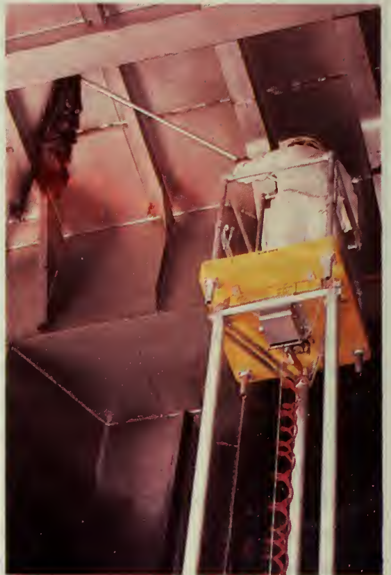
Cleaning ledges and beams of a bulk grain carrier to remove cargo residues and potential insect infestation sites.
