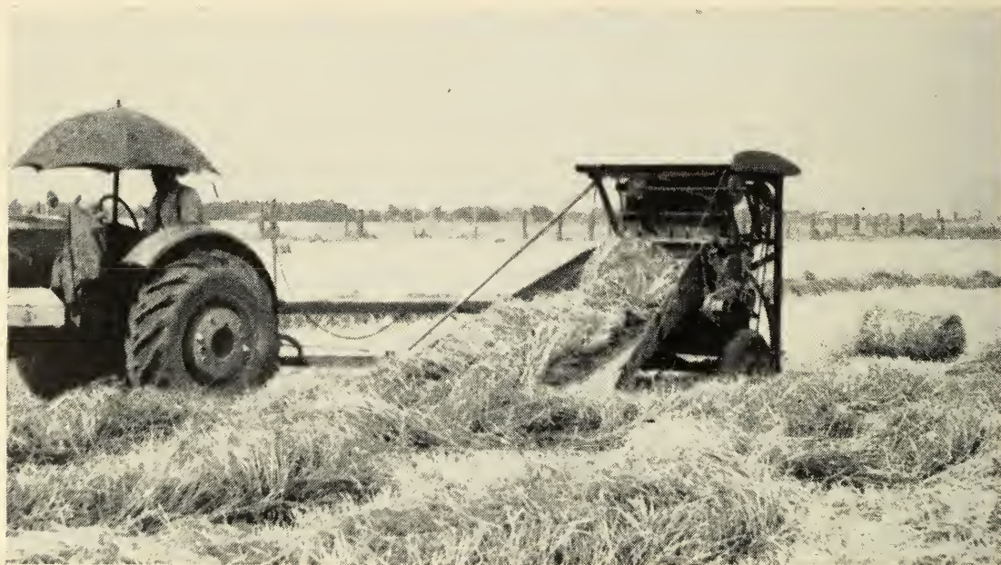
Broad throat, round bale machines can operate on a heavy windrow. As the baler is stopped to discharge each bale, a tractor with a continuous power-take-off is usually used with this baler.
