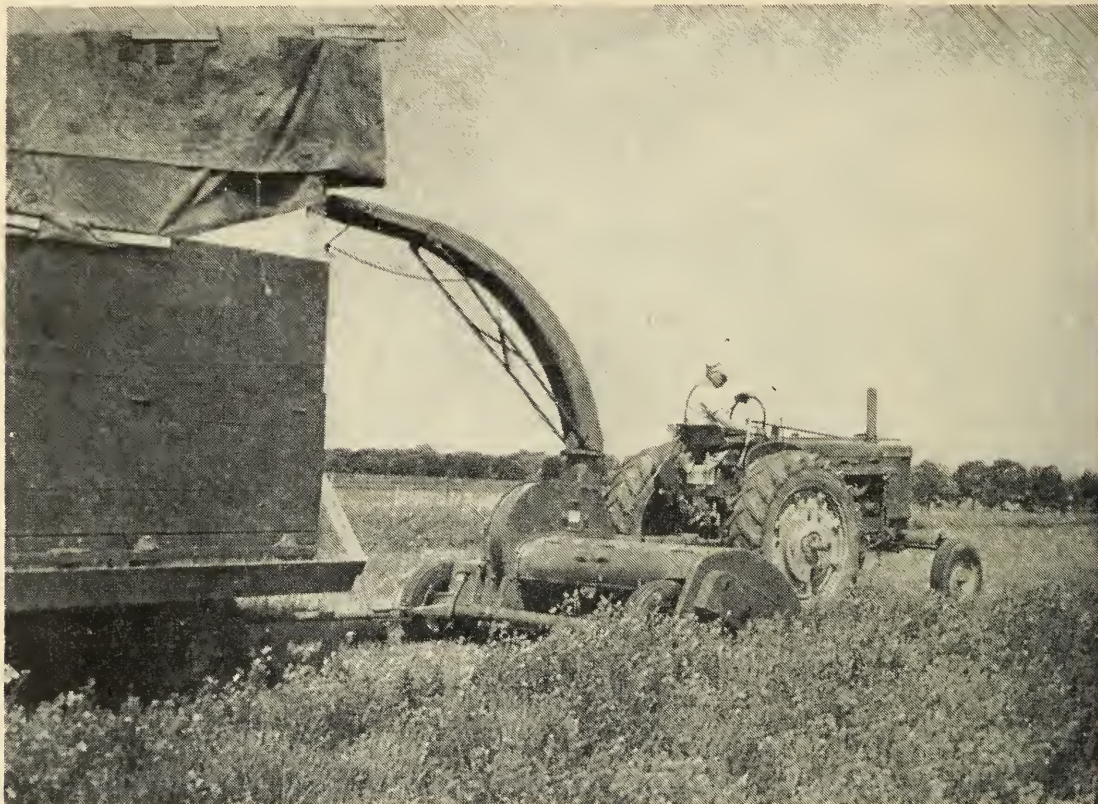
Flail harvesters shred the crop and deliver it to a wagon. This unit has an auger and blower to convey the crop from the shredder to the wagon.
