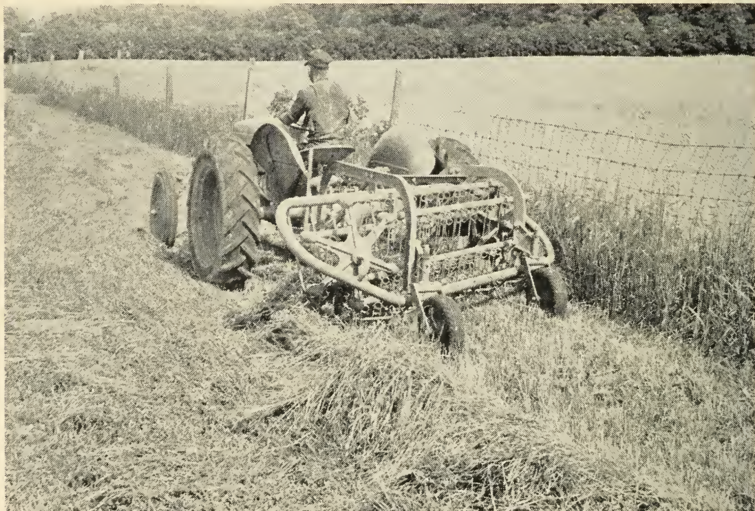
This is a roller-bar side delivery rake fitted with hydraulic lift. Since roller-bar rakes move the hay a shorter distance they tend to reduce leaf loss.
