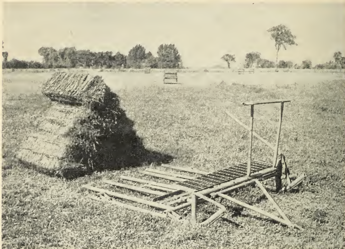
This is a bale stooker with a typical stook of bales. The bales are piled on the pipe platform by hand. An attachment for a tractor loader is available to load the stook on a wagon.
