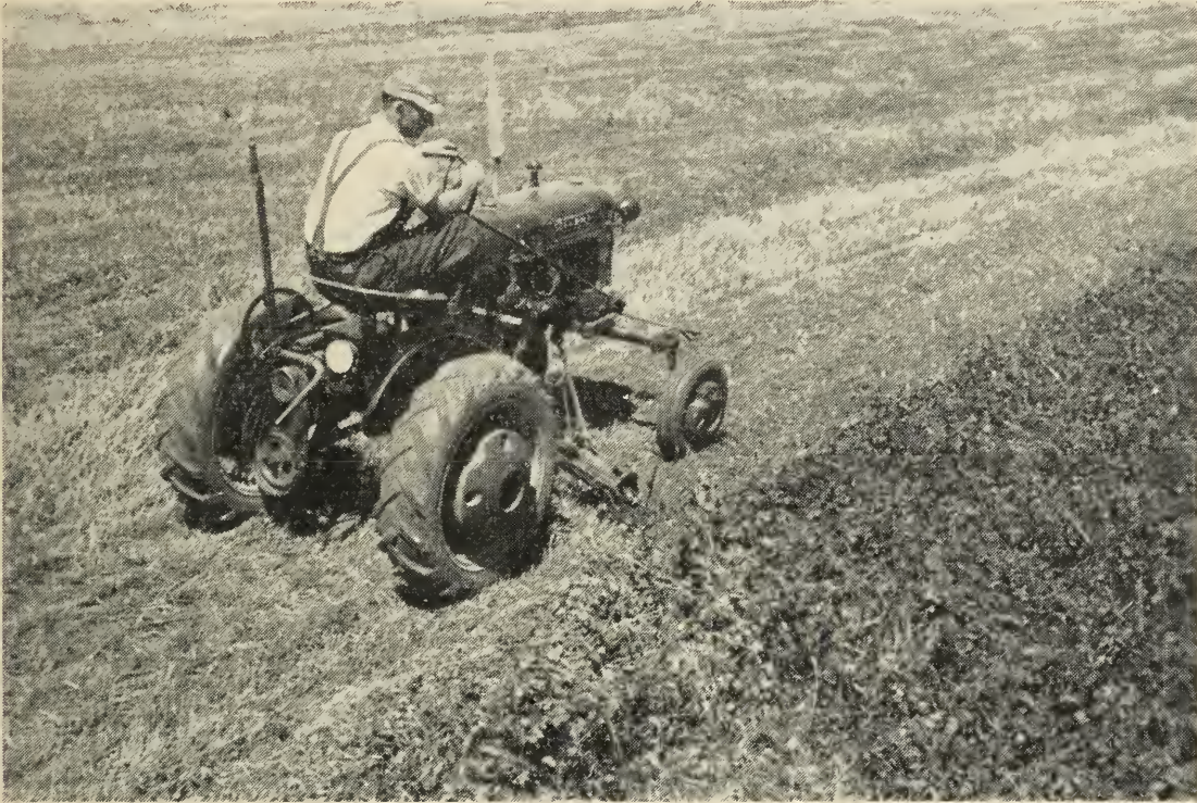
Side-mounted tractor mowers permit a clear view of the cutter bar. Hand or power operated devices are available for lifting cutter bars on tractor mowers.
