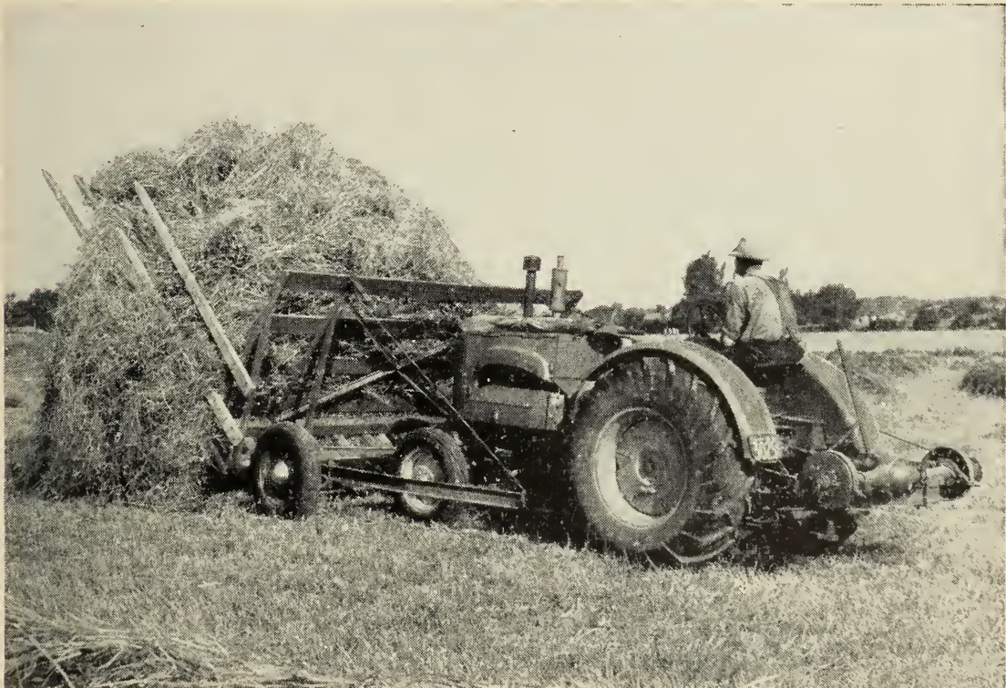
Both commercially made and homemade sweep rakes are used in harvesting. The sweep rake, where it can be satisfactorily used, eliminates heavy manual labor in gathering hay.
