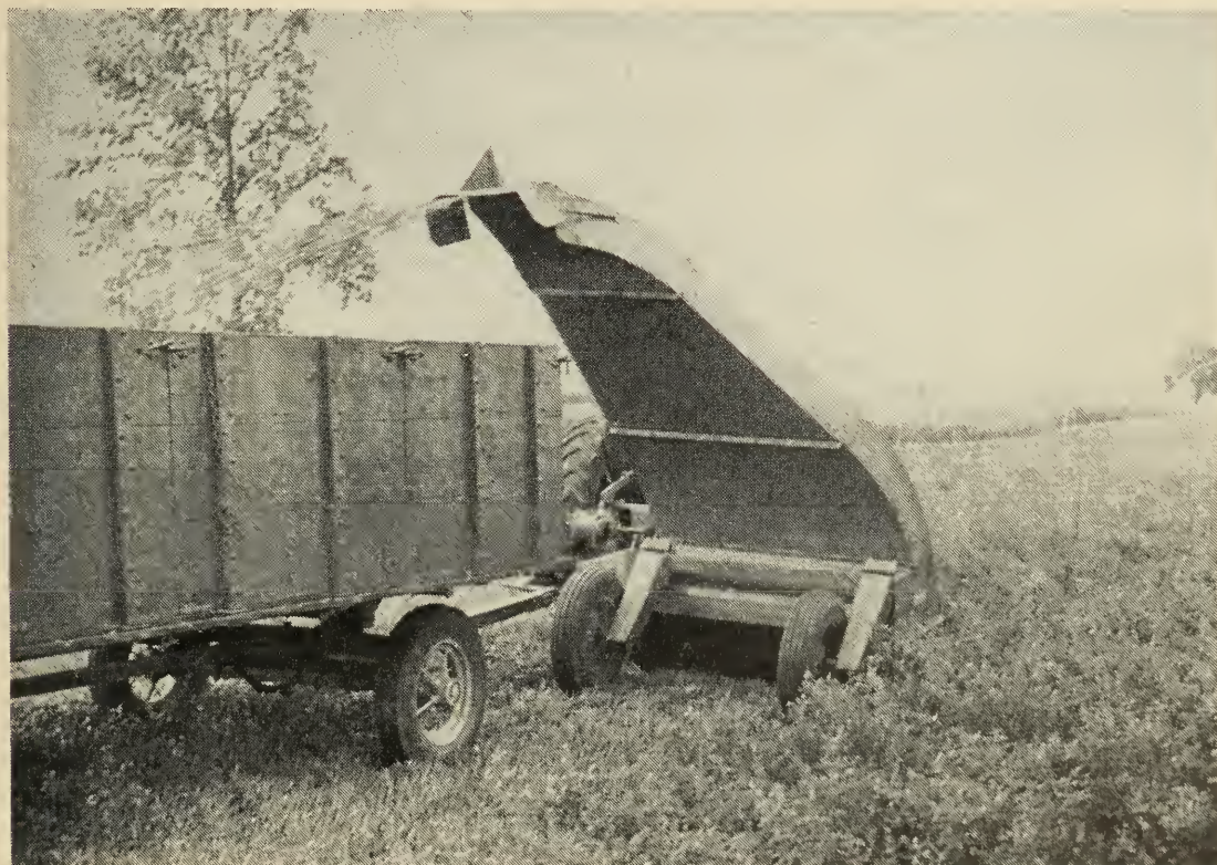
By off-setting the harvester, the standing crop is untrampled by the tractor wheels. This harvester uses a flail shredder that cuts and elevates the crop in one operation.
