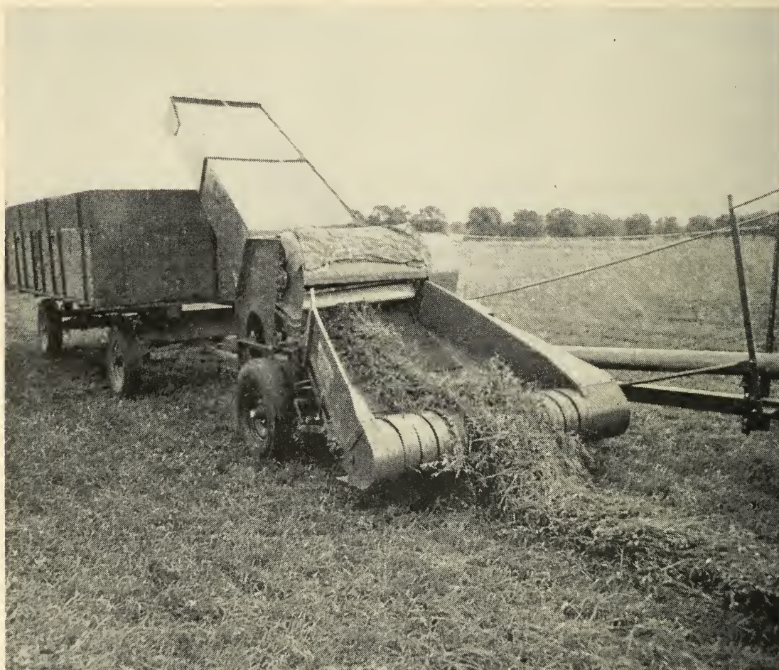
This is a new type of forage harvester. The crop is chopped as it passes between a rubber roller and knife drum and a fan blows the material into the wagon.
