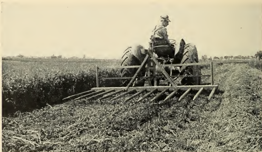
Silage sweep rakes carry loads of 400 to 700 pounds and can be used economically on a hauling distance of \frac{1}{2} mile or less. Smooth fields and good roads from the fields to the trench silo facilitate operations.
