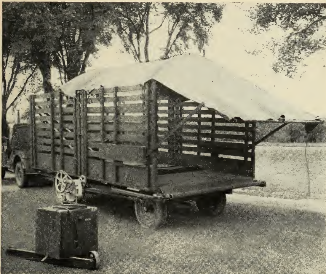
A wagon with a flat top rack, high slatted side sections, a canvas hood to retain chopped material, a hinged end gate, and a power unloader is suitable for use with forage harvesters.
