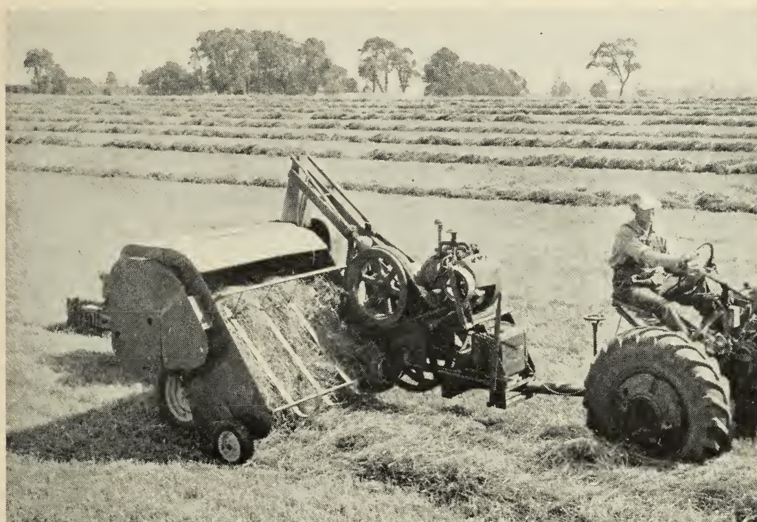
Automatic twine tying balers may be used to bale straw, hay, and similar materials. Balers with auxiliary engine are often preferred for custom work.
