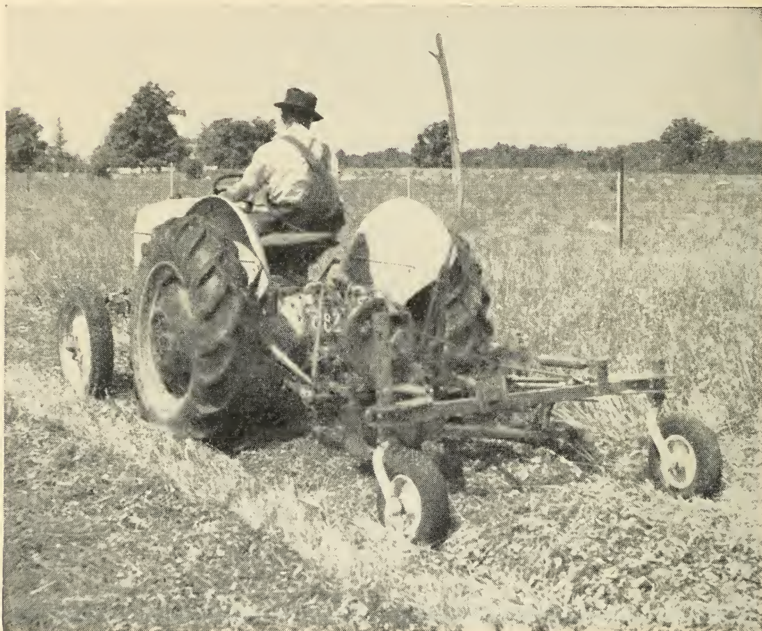
Semi-mounted mowers can be attached to practically any type and make of tractor. With a power-take-off driven cutter bar, the mower can operate at a higher speed and in heavy crops.
