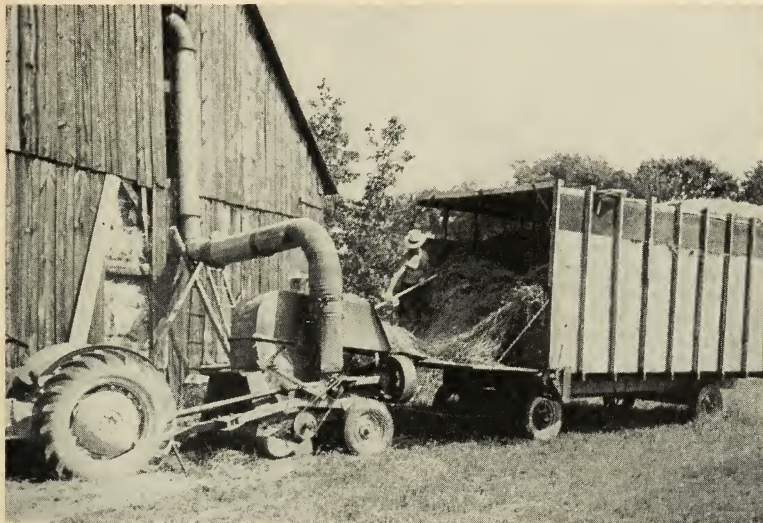
Windrowed hay may be loaded into the wagon in the field with this machine and then blown into the mow with the same equipment.
