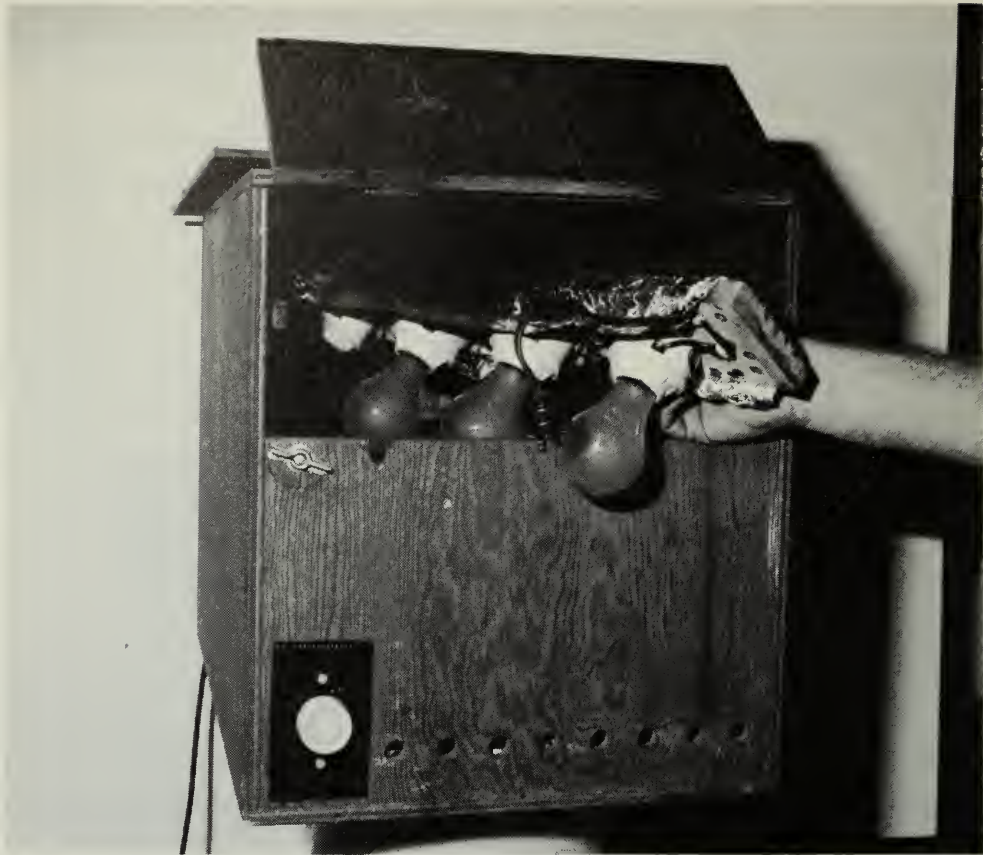
FIG. 11 A home-built cabinet dryer with light-bulb heat source (see Fig. 12 for construction details).
