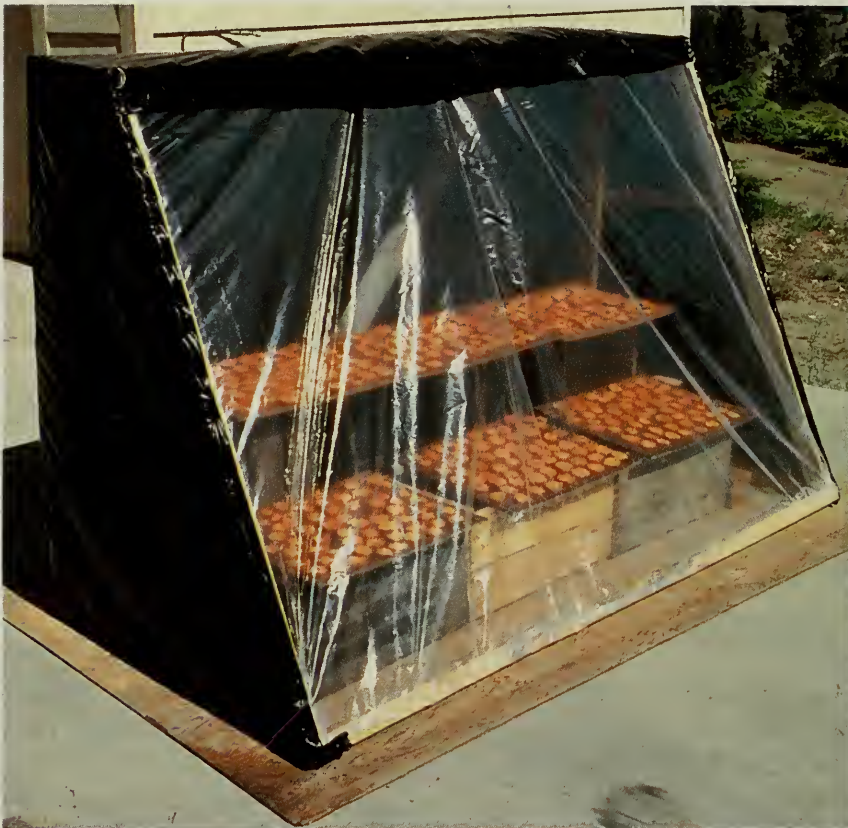
FIG. 1 A simple but effective solar dryer, with plastic cover (see Fig. 16a for construction details).
