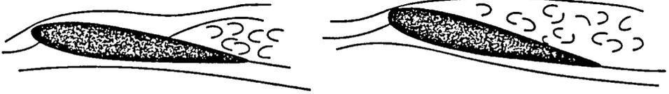
**TYPE II - DÉCROCHAGE AVEC DÉCOLLEMENT AU BORD D'ATTAQUE**
