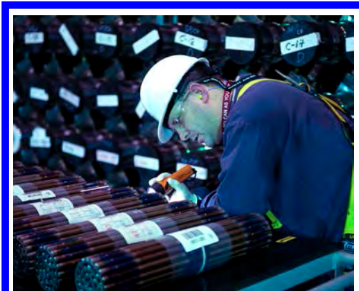
Inspection of new fuel bundles, before they are inserted into the reactor.
