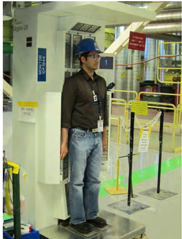
A CNSC inspector uses a whole-body monitor to detect radiation levels. This precautionary measure is used at NPPs, to ensure that no radioactive contamination is spread outside of the premises by workers or inspectors.
