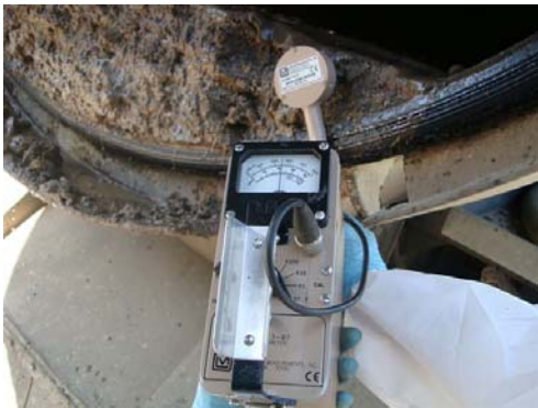
Survey meter detecting NORM in the sludge of a contaminated vac truck (Photo courtesy of Tervita Corporation)
