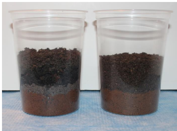
Figure 2 Test units showing layering of soil horizons: (L) an Ontario podzol (Ah, Ae, and B horizons) and (R) a Saskatchewan brunisol (FH and AeB horizons) (photo: H. Lemieux)
