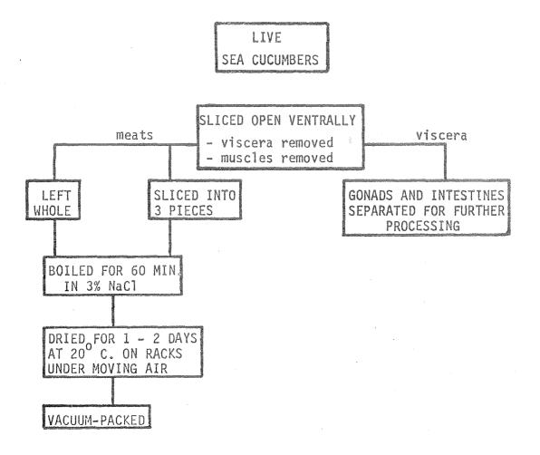
Figure 6. - Flow diagram of drying process for Dried Sea Cucumber (DSC).
