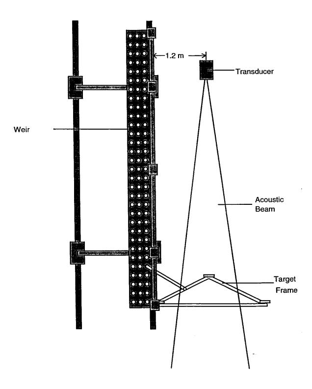
Fig. 6: Top-down view of the weir with target frame attached. This is the configuration used during standard target calibrations.
