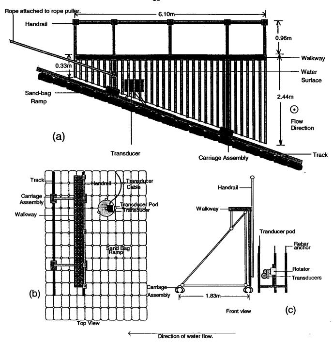
Fig. 3: Side (a), top (b), and front (c) schematic views of the diversion weir and track.
