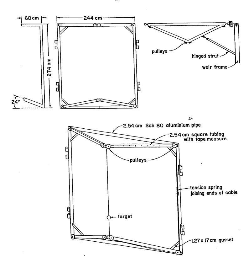
Fig. 4: Side, front, top, and three-dimensional views of the target frame.
