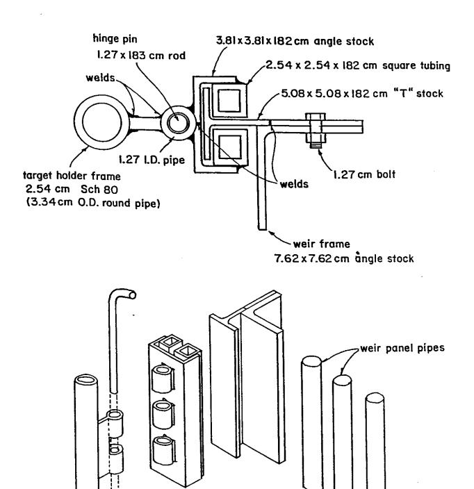
Fig. 5: Hinge and slide receiver connecting the target frame to the weir.
