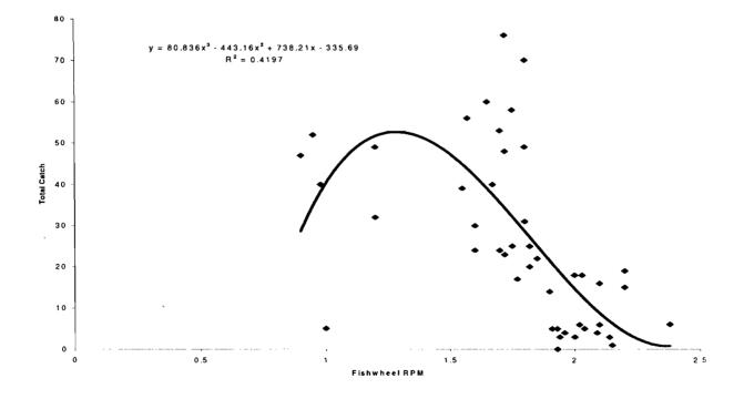
Figure 7b. Fishwheel rotational speed related to total catch, Klinaklini River, 1999.
