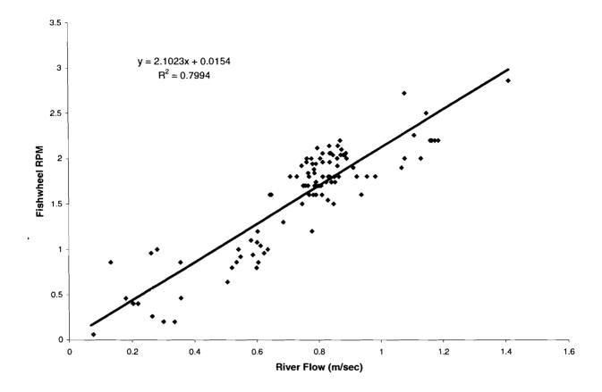
Figure 6. Fishwheel rotational speed related to water flow, Klinaklini R., 1999.
