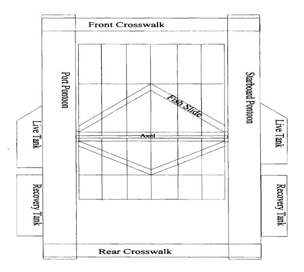
Figure 3. Schematic diagram of fishwheel (aerial view).
