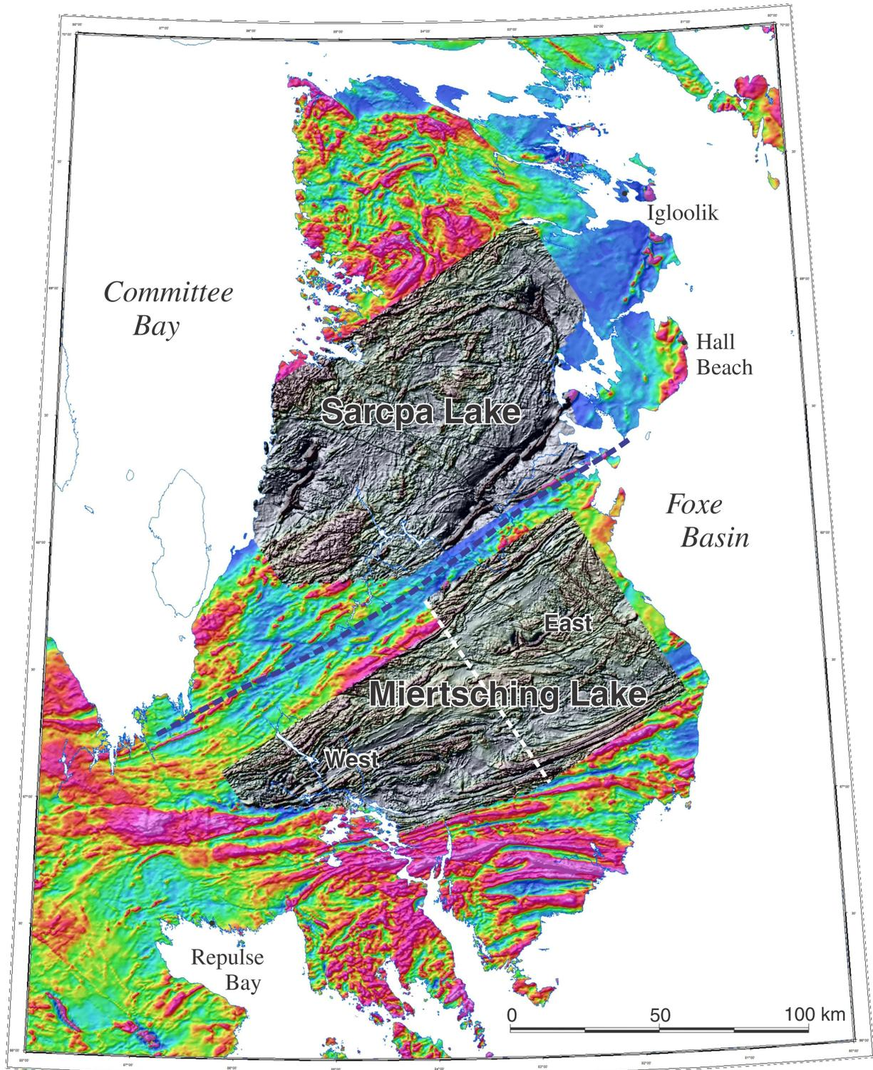
**Figure 3. a)** Map of Melville Peninsula with total-field aeromagnetic images from three new high-resolution surveys (Sarcpa Lake, West Miertsching, East Mertching), shown in shaded relief. Line spacing: 400 m, flight height: 150 m. The regional aeromagnetic image in background is from analogue acquisition from the 1970s. The boundary separating the 'northern structural zone' from the 'southern structural zone' is shown (blue dashed line, see text for explanation).
