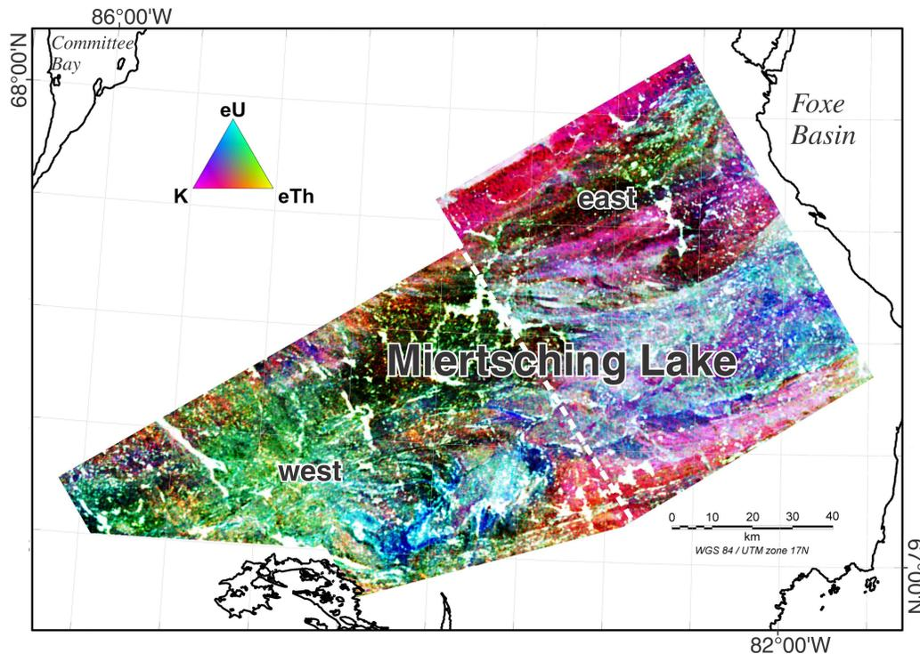
**Figure 3. (cont.) b)** High-resolution (see Fig. 3a) airborne radiometric map, Miertsching Lake survey, with ternary U-K-Th plot shown.
