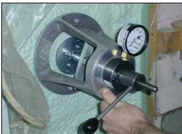
Figure 1 Device used to test tear strength force
