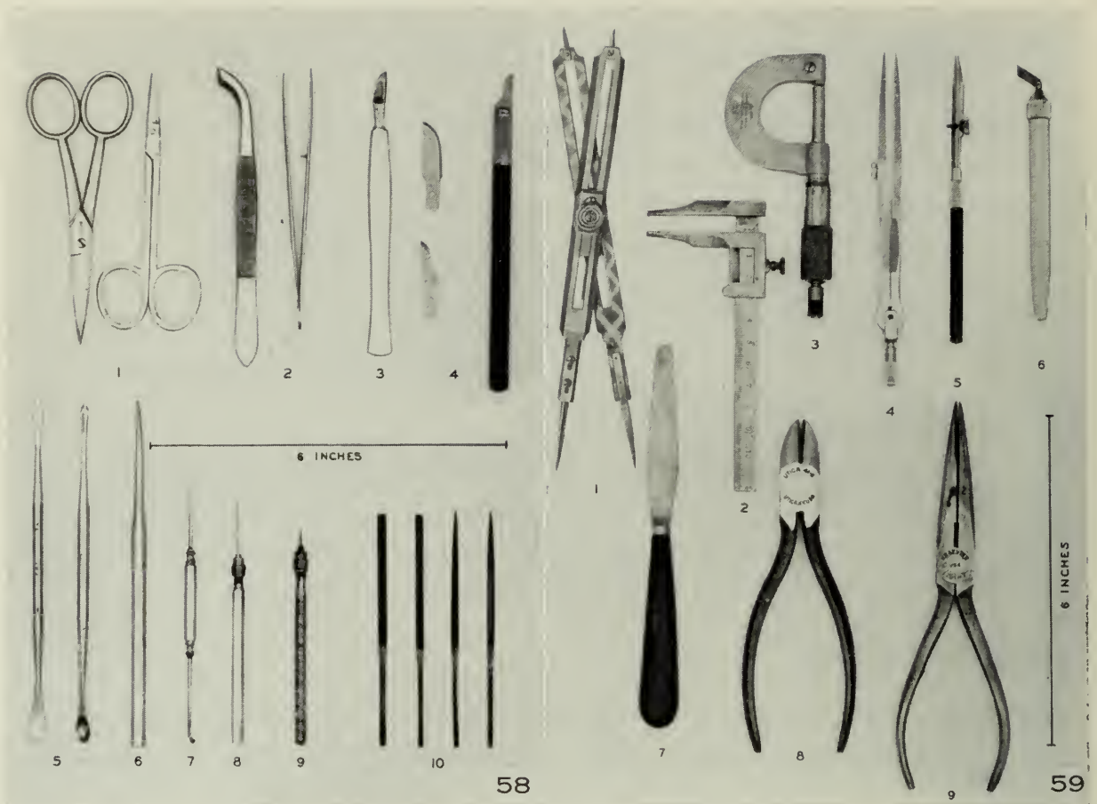
Figure 58 —(1) Scissors, (2) forceps, (3) scalpel, (4) combination knife, (5) wax spatulas, (6) dental probe, (7) spoon and seeker, (8) dissecting needle, (9) holder for razor-blade splinter, (10) Swiss pattern files.
