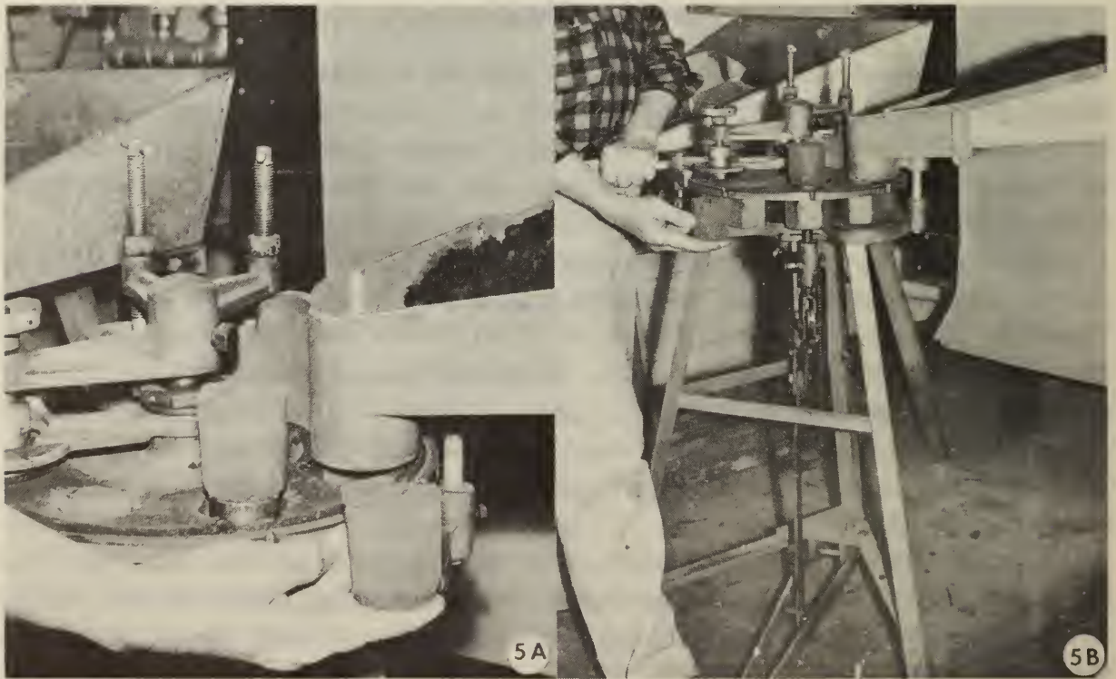
Figure 5a. - Close-up of soil blocks made by the 'Quick Press' blocking machine.
