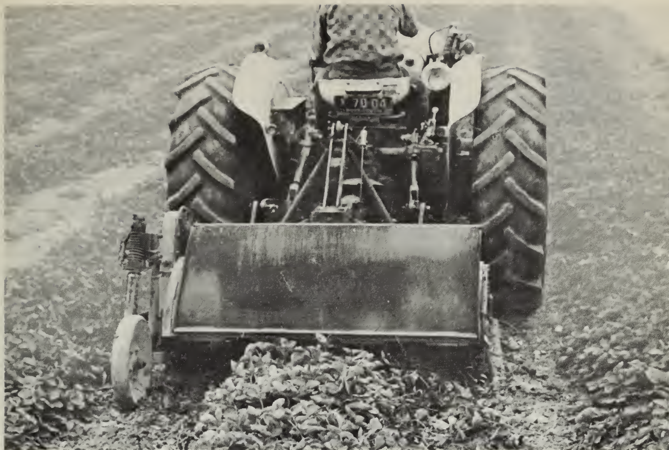
Fig. 15 Renovating the field with a rotary-type tiller.
