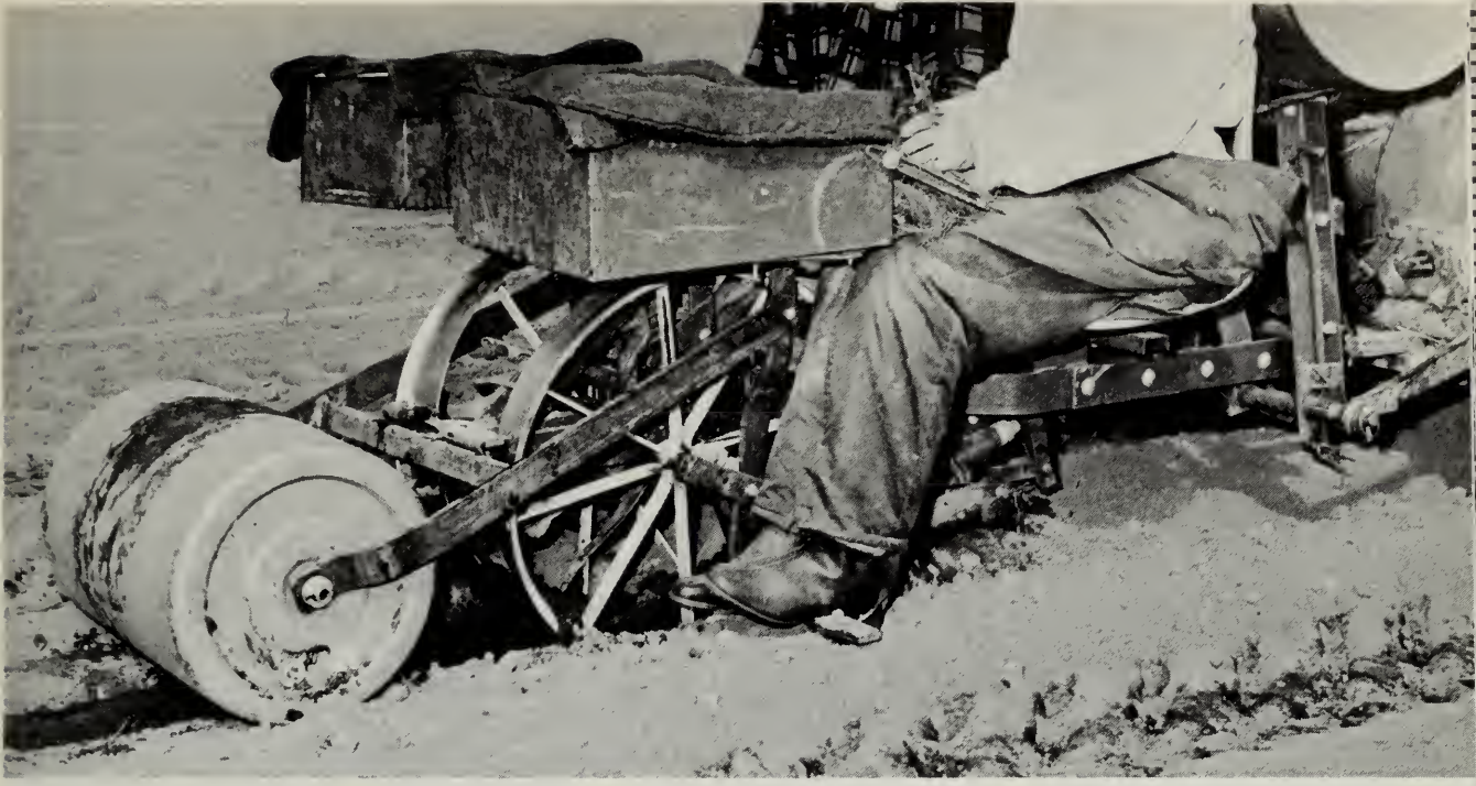
Fig. 4 A mechanical transplanter reduces planting time and provides water for the newly set plants.
