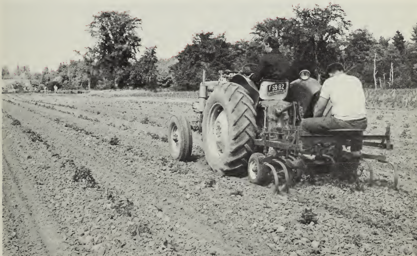
Fig. 7 A tractor-mounted wiggly hoe is a very useful piece of cultivation machinery
