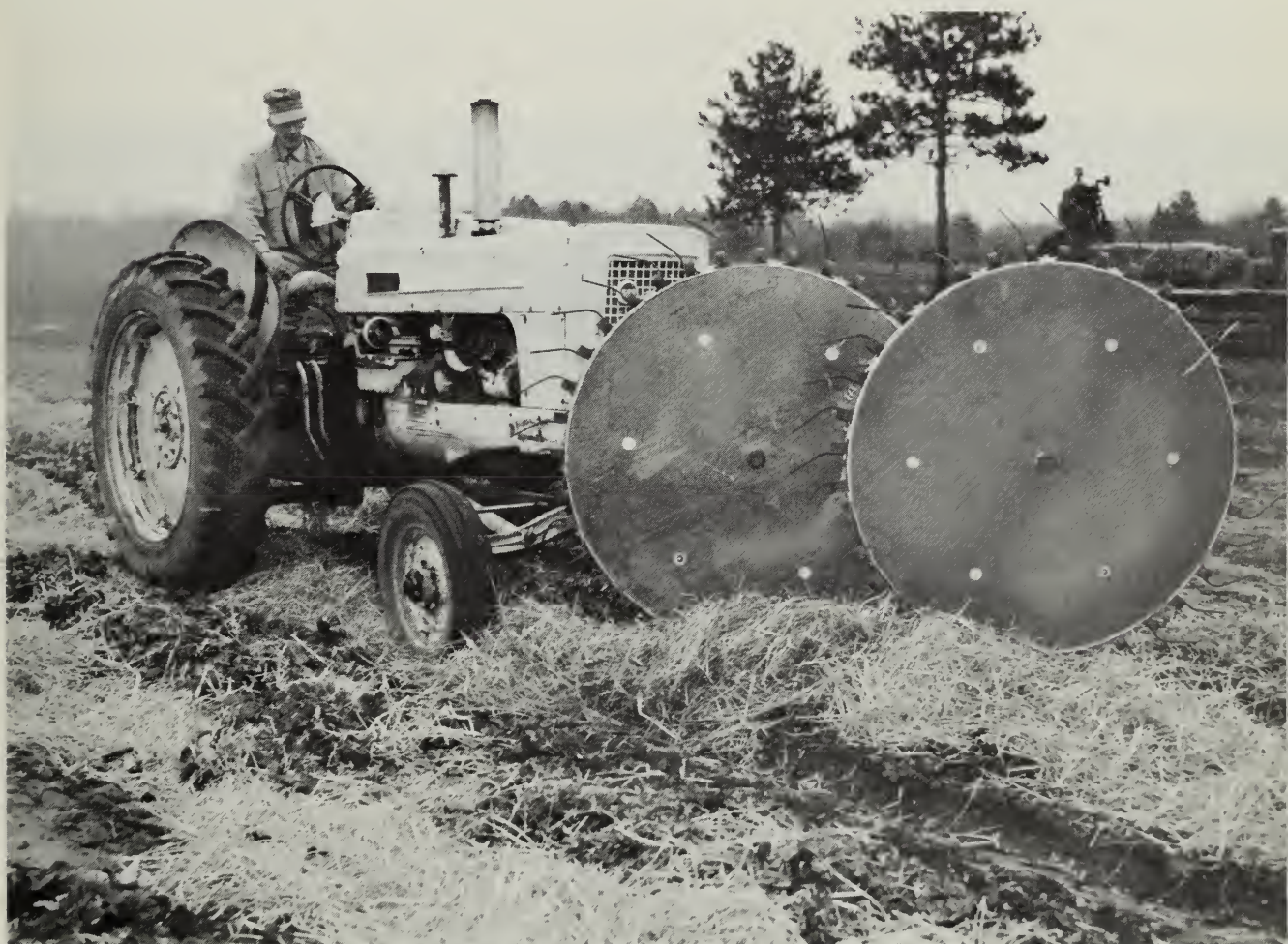
Fig 9 A rig to remove the straw from the plants.
