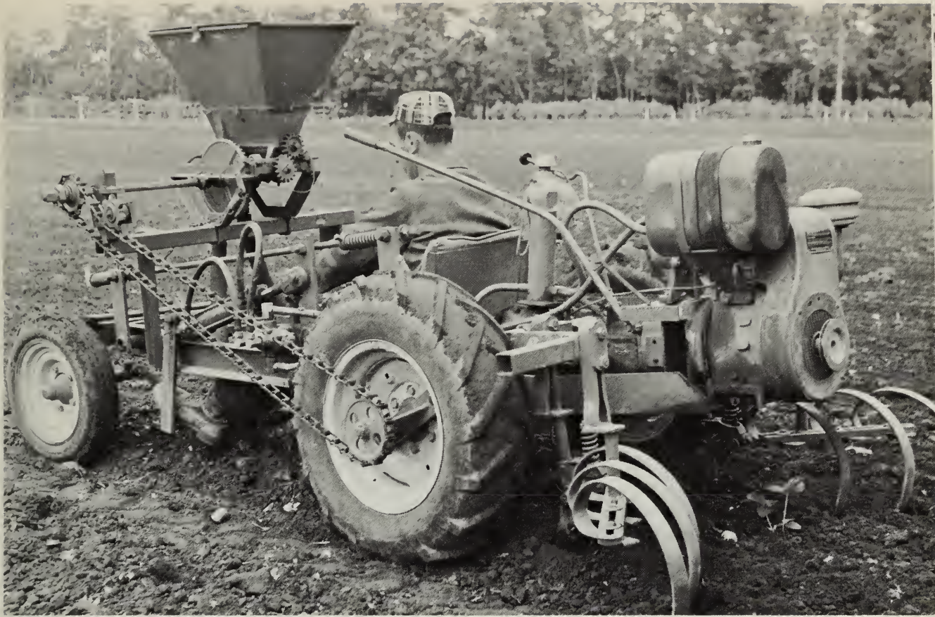
Fig. 6 A self-propelled cultivator is guided by your feet, leaving your hands free to operate a pair of wiggly hoes. Fertilizer can also be applied with this machine.
