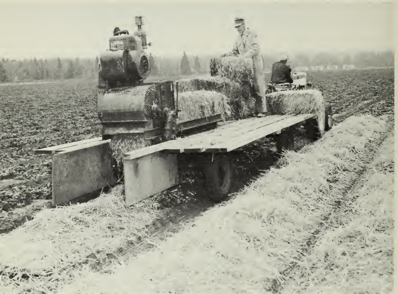
Fig. 8 A straw shredder is used for mulching large areas.
