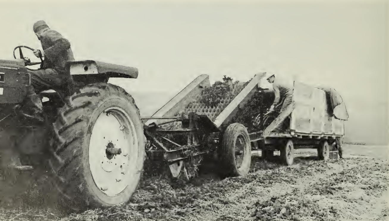
Fig. 1 Mechanical digger used by nurserymen to harvest plants.
