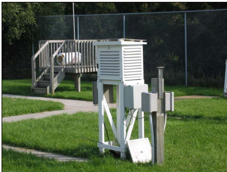
Weather stations, such as the Stevenson screen above, measure air temperature and contribute to daily observations used in the NRT data system.
