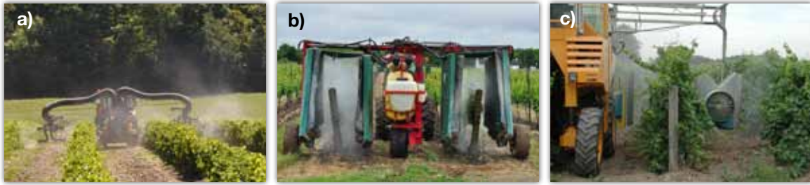
Fig. 60: Pesticide spraying in a vineyard: a) airblast sprayer in Quebec; b) recycling sprayer in Ontario (Photo Queen's Printer for Ontario 2015. Reproduced with permission; c) airblast sprayer in Ontario (Photo Wendy McFadden-Smith).
